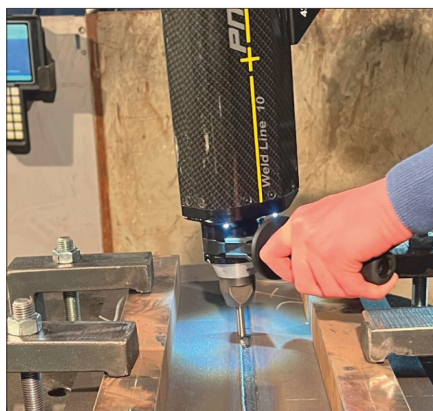
Fig. 4. Test plate during peening
