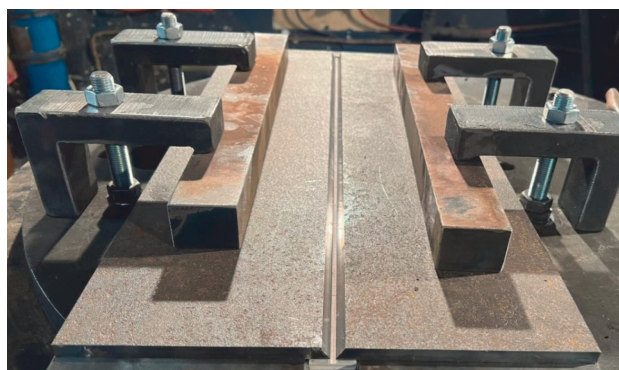
Fig. 2. Test plate with the ceramic backing strip on the welding robot table
