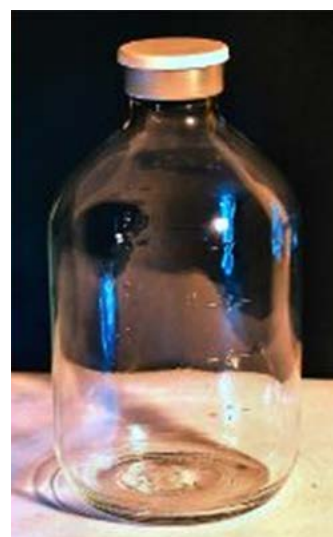
Fig. 5: EMPT crimping of a sterile aluminium lid onto a pharmaceutical glass bottle
