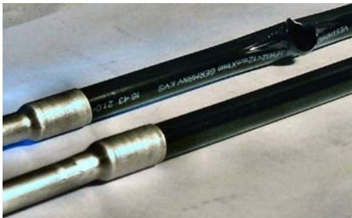
Fig. 3: EMPT crimping of steel fittings onto rubber hoses
