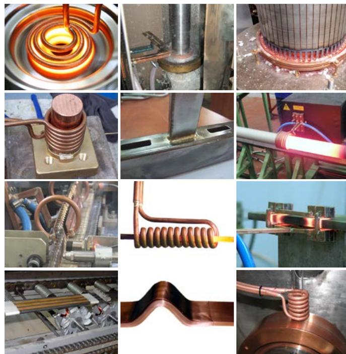
Fig. 2. Examples of induction heating applications: surface hardening, brazing, coat remelting, stress relief annealing, heating before forging, rotor soaking after varnishing, induction welding of sheets, production of amorphous and nanocrystalline strips.
