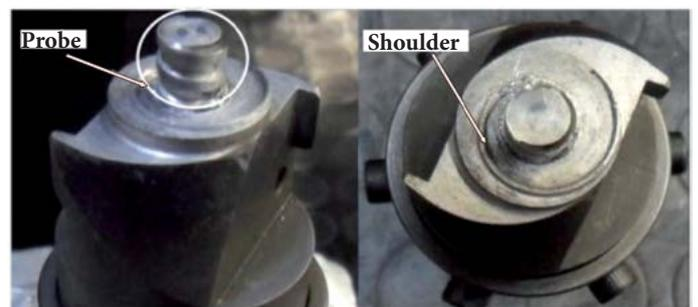
Fig. 12. Tool used to produce the curing mould prototype
