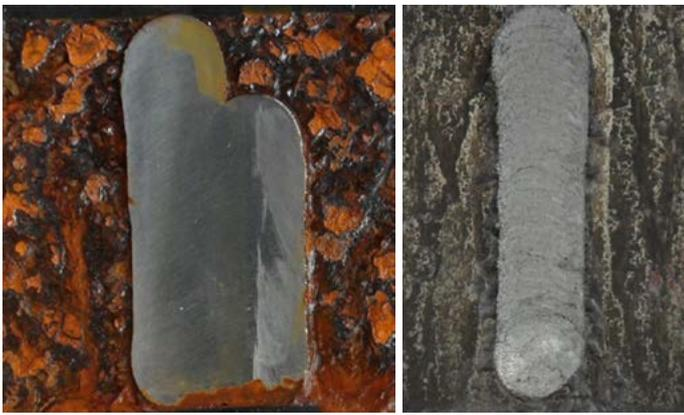
Fig. 4. Case study on corrosion properties: Stainless steel on mild steel (left) and AA6082 on AA2024 (right)
