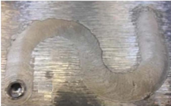
Fig. 13. Prototype with serpentine profile
