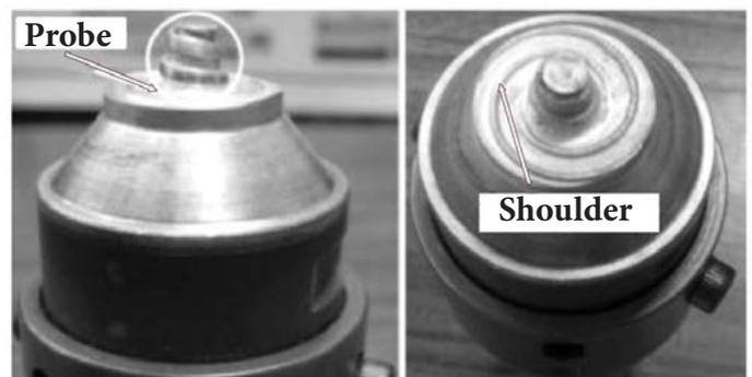
Fig. 8. Tool used to produce the injection mould prototype
