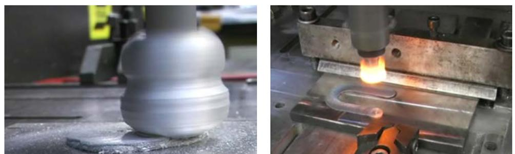
Fig. 6. Possibilities of the application of Friction Surfacing: build up (left) and conformal coatings (right)
