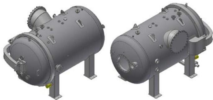
Fig. 2. Pressure vessel model (without simplified representations) for numerical calculations
