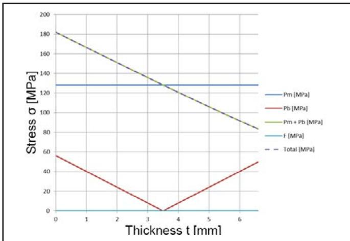
Fig. 5. Linearization of stress in the SCL1 zone (Fig. 4) in the area critical for the welded joint according to Figure 1-D1 (shell-nozzle branch joint)
