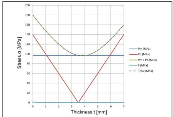
Fig. 7. Linearization of stress in the SCL2 zone (Fig. 6) in the area critical for the welded joint according to Figure 1-D1 (shell-nozzle branch joint)
