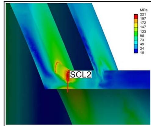
Fig. 6. Location of stresses in the SCL2 zone (see area in Fig. 3a)
