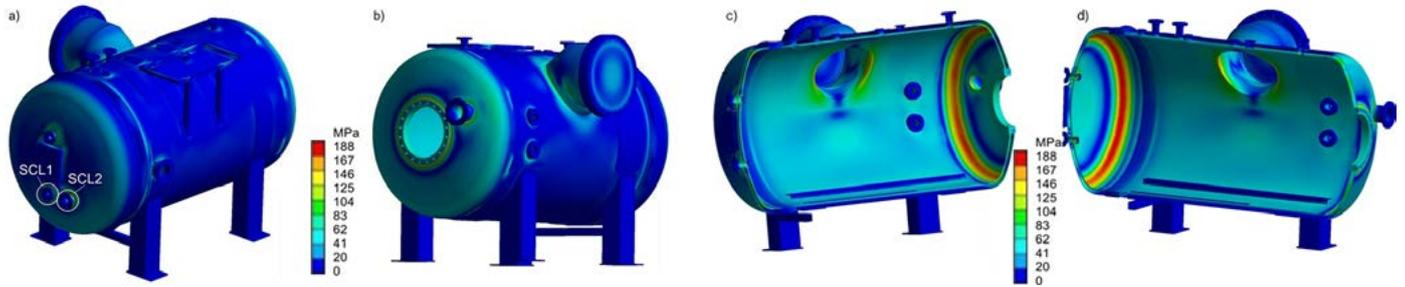
Fig. 3. Distribution of reduced stresses according to the von Mises hypothesis in the pressure vessel designed: front view (a) and rear view (b) and cross-sectional views (c and d)
