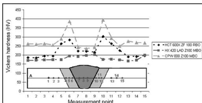
Fig. 2. Hardness measurement results for selected butt joints made of the HCT 600X ZF 100 RBO, HX 420 LAD Z100 MBO and CPW 800 Z100 MBO steels
