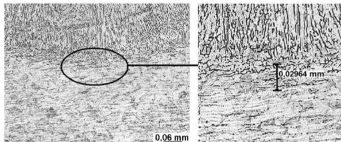
Fig. 4. Microstructure of the overlay weld made of the X5CrNi18-10 steel with 60% EN ratio, electrolytic etching
