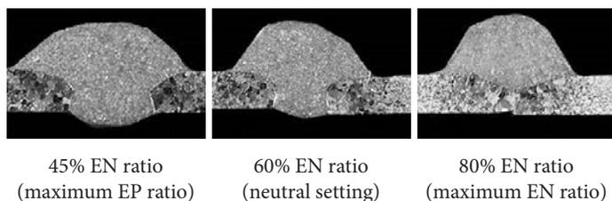
Fig. 9. Macrostructure of the joints made of the 1 mm thick X6CrTi17 steel, mag. 5.0x, etching with Adler's reagent
