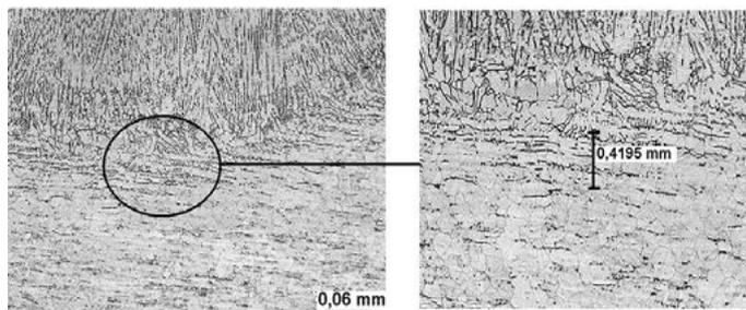
Fig. 6. Microstructure of the overlay weld made of the X5CrNi18-10 steel with 45% EN ratio, (maximum EP ratio), mag. 200x, electrolytic etching
