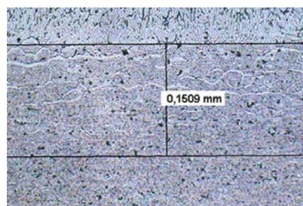
Fig. 13. Microstructure of the overlay weld made with 45% EN ratio setting, mag. 200x, etching with Keller's reagent
