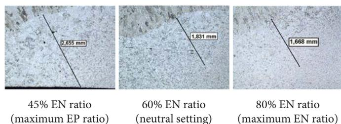
Fig 1. Microstructures of overlay welds made with various EN ratio settings in current waveform with HAZ widths marked, magnification 25 x, etching Nital
