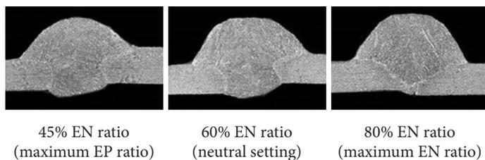
Fig. 7. Macrostructure of the joints made of the 1 mm thick X5CrNi18-10 steel welded with various EN ratio settings in the current waveform, mag. 5.0x. etching with Adler's reagent
