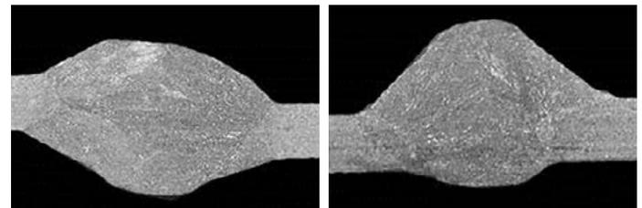
Fig. 8. Macrostructure of the joints made of the 1 mm thick X5CrNi18-10 steel welded with the standard arc, mag. 5.0x. etching with Adler's reagent
