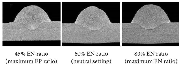
Fig. 3. Macrostructure of the overlay welds made of the 2 mm thick X5CrNi18-10 steel, mag. 5.0x. etching with Adler's reagent
