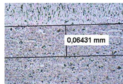
Fig. 14. Microstructure of the overlay weld made with 80% EN ratio setting, mag. 200x, etching with Keller's reagent
