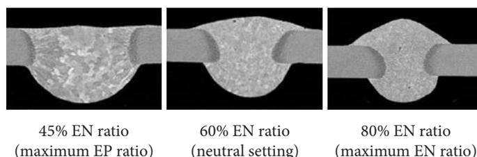
Fig. 15. Macrostructure of the joints welded using the synergic line and various EN ratio settings, etching with Keller's reagent
