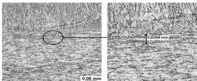
Fig. 5. Microstructure of the overlay weld made of the X5CrNi18-10 steel with 80% EN ratio, (maximum EN ratio), mag. 200x, electrolytic etching
