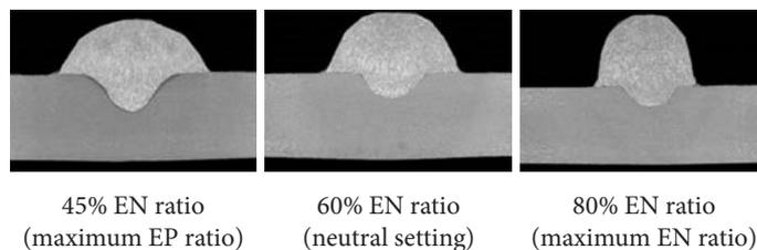
Fig. 11. Macrostructure of the overlay welds made using the synergic line with adjustable EN ratio in the welding current waveform. Welding current: 100 A, arc voltage between 15.5 V and 23.0 V, etching with Keller's reagent
