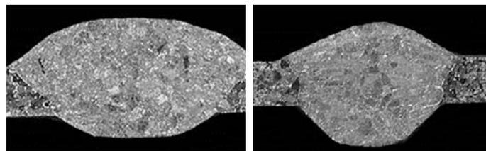
Fig. 10. Macrostructure of the joints of the 1 mm thick X6CrTi17 steel made using VP welding variant (a) and the standard arc (b), mag. 6.0, etching with Adler's reagent
