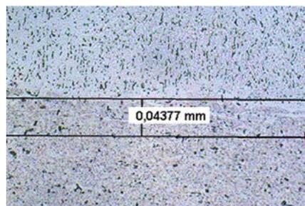
Fig. 12. Microstructure of the overlay weld made with 60% EN ratio setting, mag. 200x, etching with Keller's reagent
