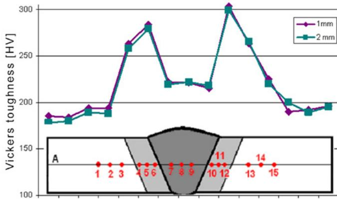
Fig. 6. Hardness measurement results for 1mm and 2mm-thick butt joints
