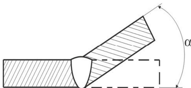
Fig. 1. Joint angular deformation
