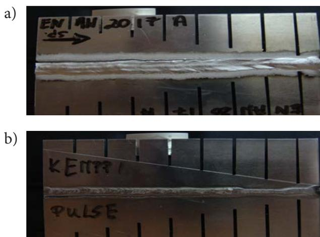
Fig. 2. Result of Houldcroft test carried out with MIG-Pulse method a) face; b) root
