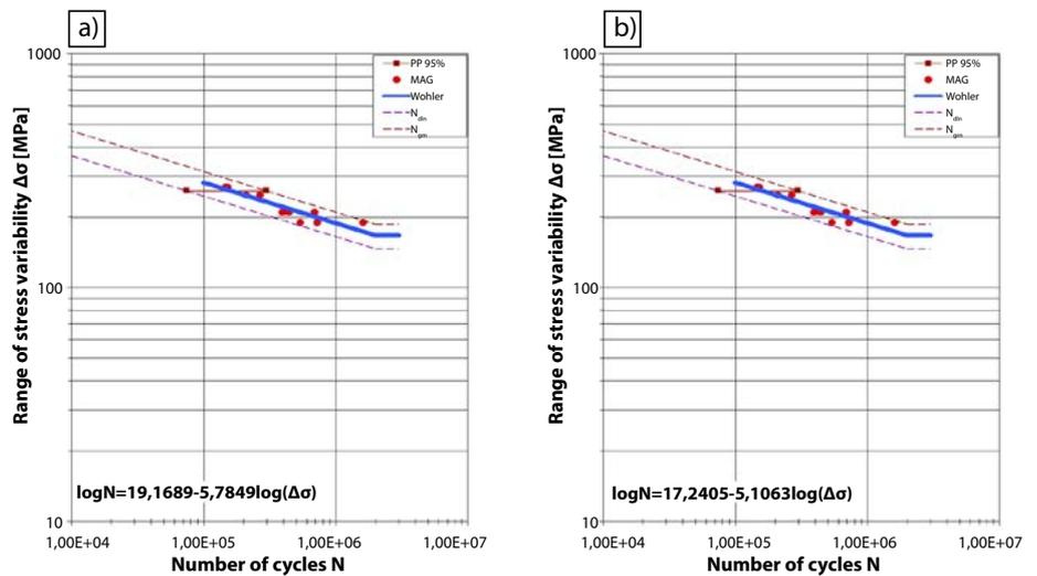
Fig. 11. Wöhler line for joint with transverse rib with fillet welds: a) without stress relief annealing, b) after stress relief annealing [19]
