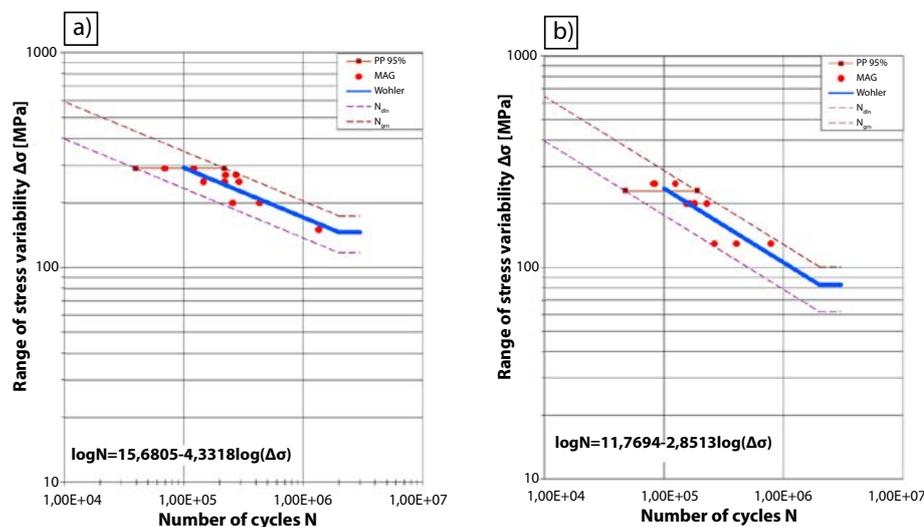
Fig. 9. Wöhler line for butt joint: a) without stress relief annealing, b) after stress relief annealing [19]
