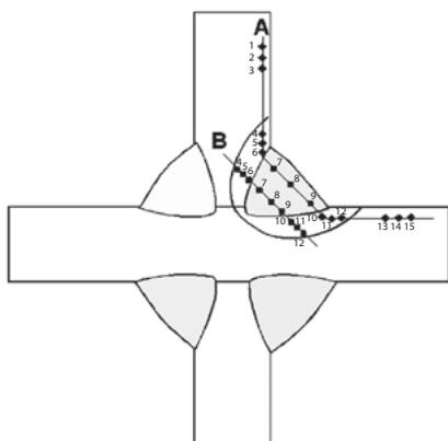
Fig. 4. Arrangement of hardness measurement points in S420MC steel cruciform joint with fillet welds [19]
