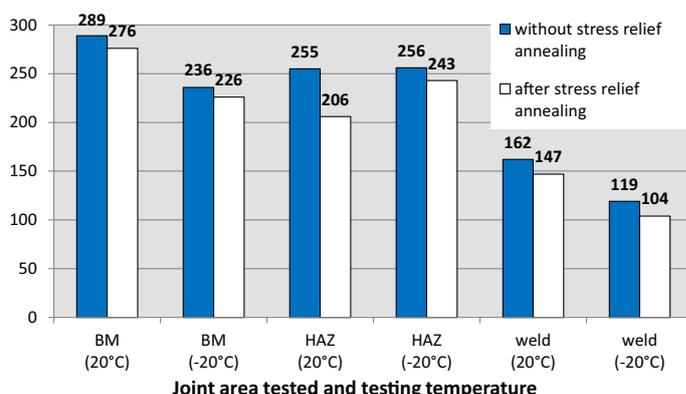
Fig.3. Impact energy test results for S420MC steel welded joints [19]
