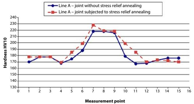
Fig. 5. Hardness distribution of S420MC steel welded joints without and after stress relief annealing [19]
