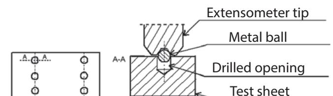
Fig. 6. Sketch of preparing measurement point in test sheet with welded joint [19]
