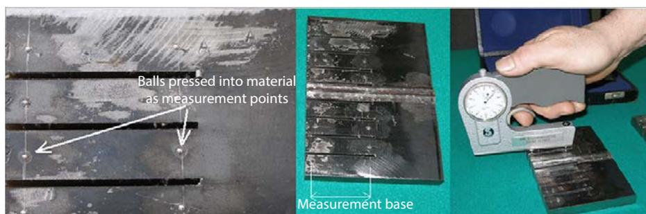
Fig. 7. Butt welded joint test elements for measuring internal stresses and manner of measurement with mechanical extensometer [19]
