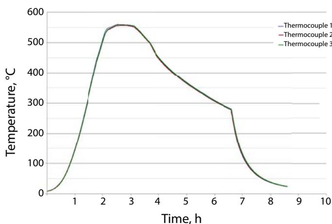
Fig. 1. Diagram of stress relief annealing process [19]
