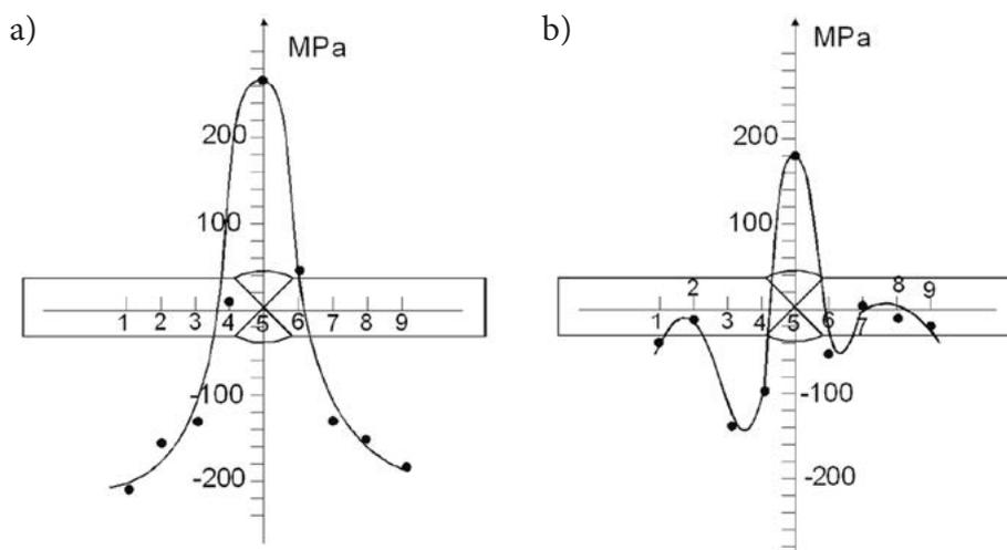
Fig. 8. Distribution of internal stresses in S420MC steel butt joint; a) without stress relief annealing, b) after stress relief annealing (stress values according to Table no. 3) [19]
