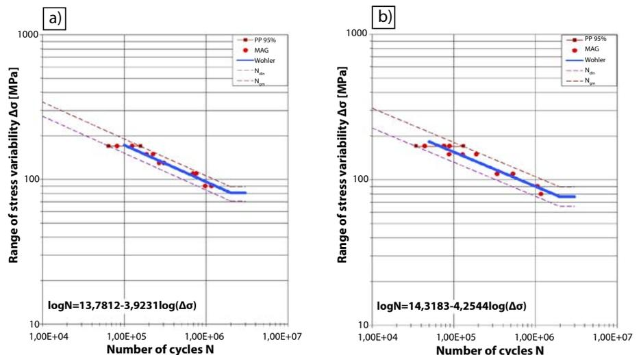
Fig. 12. Wöhler line for cruciform joint with fillet welds: a) without stress relief annealing, b) after stress relief annealing [19]
