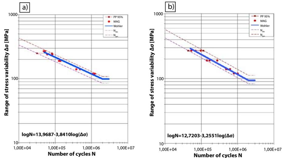
Fig. 10. Wöhler line for joint with longitudinal rib with fillet welds: a) without stress relief annealing, b) after stress relief annealing [19]
