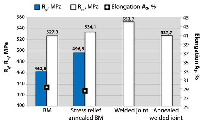
Fig. 2. Mechanical properties of base metal and of S420MC steel welded joints [19]
