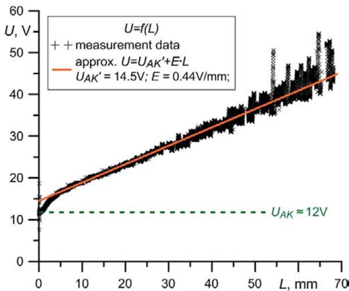
Fig. 5. Gradient characteristic of the electric arc subjected to tests
