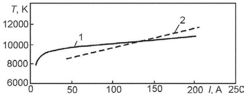
Fig. 2. Dependence of plasma temperature on TIG welding arc current (1, 2 – approximations of various data by various authors)
