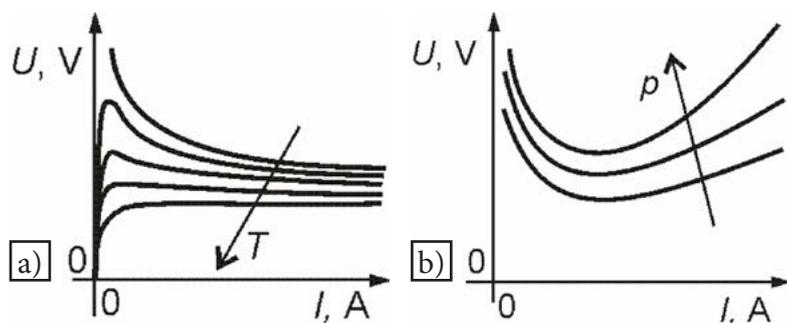
Fig. 4. Arc static voltage–current characteristics: a) in gas of various temperatures; b) in gas of various pressures
