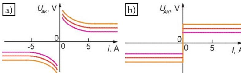
Fig. 3. Approximations of near-electrode voltage drop characteristics a) for low-current arcs and b) high-current arcs
