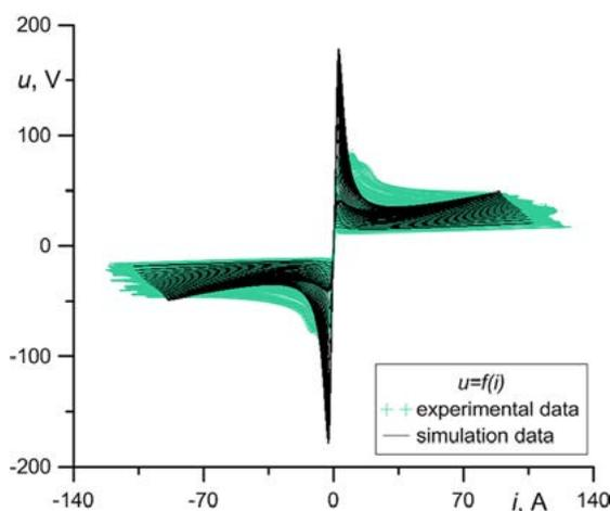
Fig. 8. Dynamic characteristics of experimentally tested arc and simulated arc during tension
