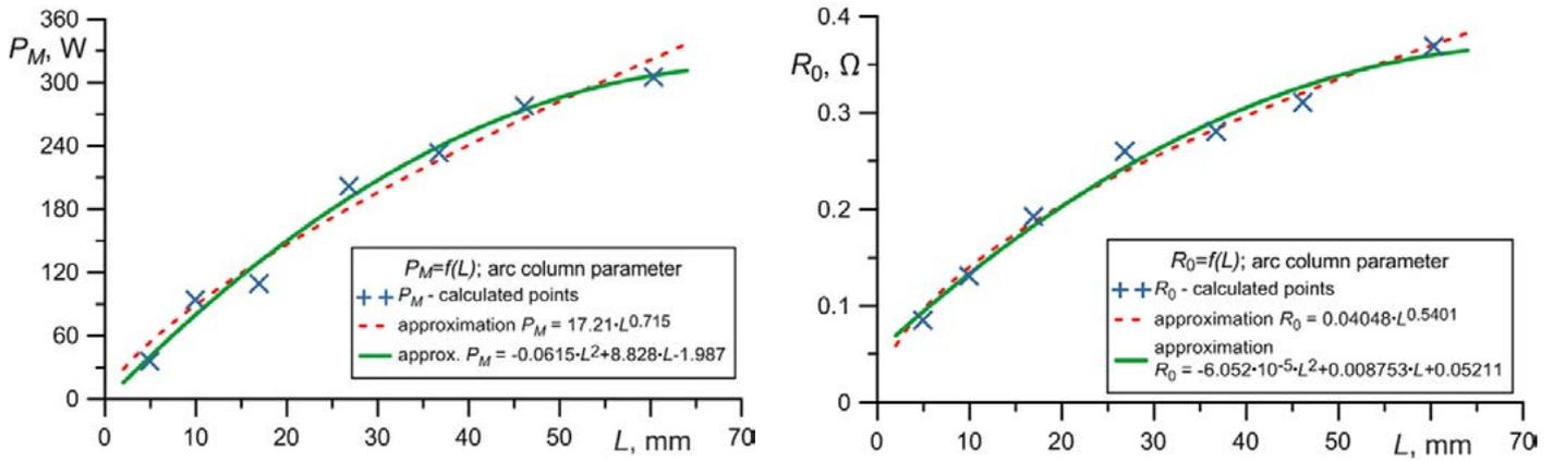
Fig. 6. Approximations of arc column parameters: a)  $P_M=f(L)$ ; b)  $R_0=f(L)$
