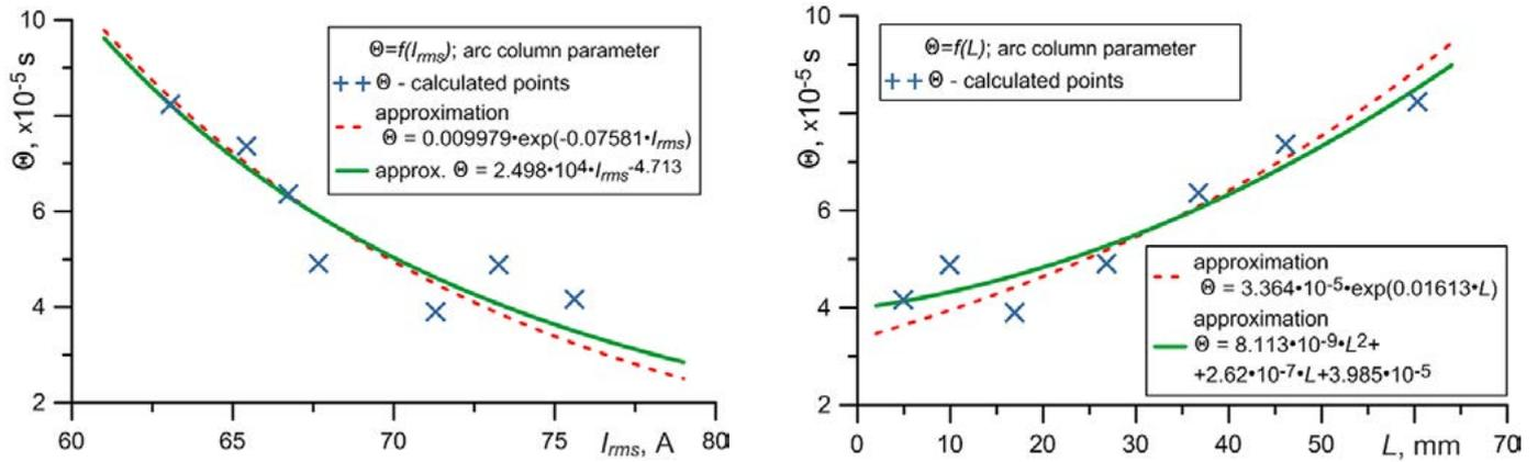
Fig. 7. Approximation of arc model time constant: a)  $\theta=f(I_{rms})$ ; b)  $\theta=f(L)$
