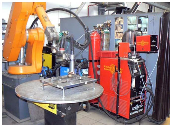
Fig. 2. Plasma welding station equipped with the Romat 310M welding robot manufactured by Cloos and the Eutronic GAP 3001 welding machine manufactured by Castolin
