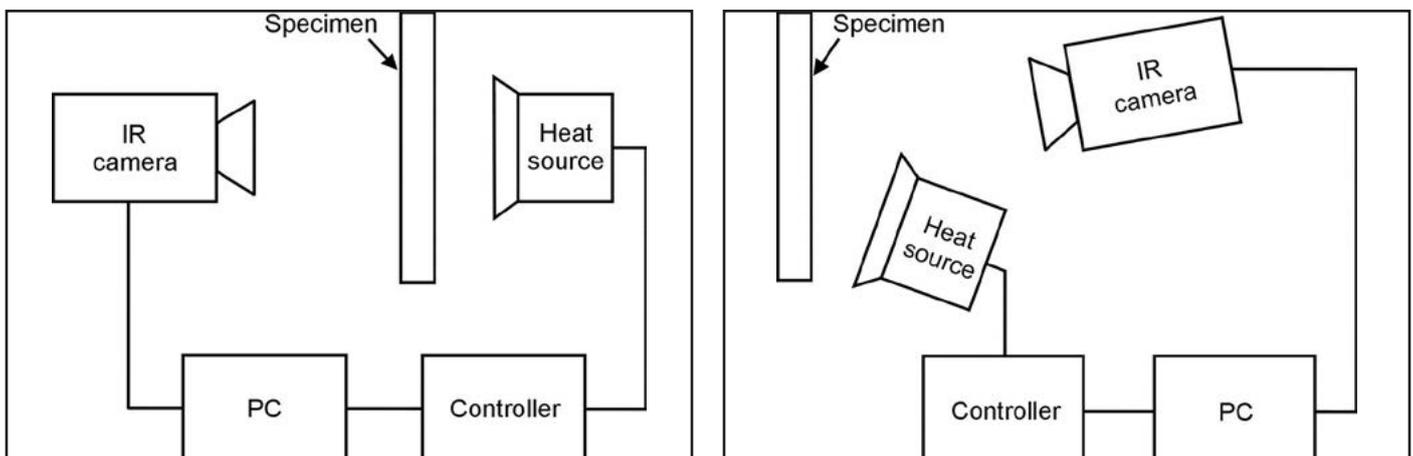
Fig. 2. Schemes for active thermography experimental setups: a) double-sided, b) single-sided
