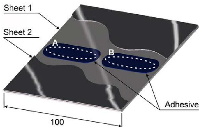
Fig. 3. Model of adhesively bonded sheet metal overlap joint with section of upper sheet 2, with specified fields (A and B) for applying adhesive
