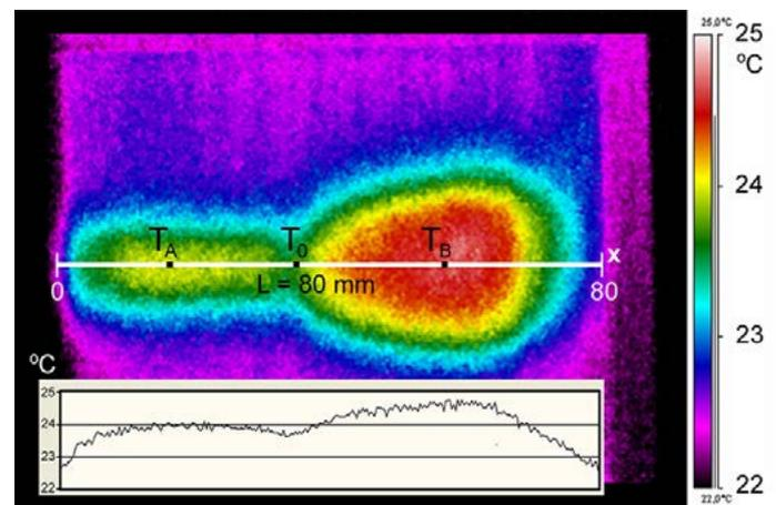
Fig.7. Thermographic image of the surface of specimen 4 with the momentary temperature profile along the straight line representing the location of the adhesive layer axis
