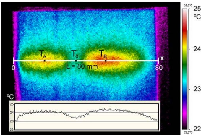
Fig. 4. Thermographic image of the surface of specimen 1 with the momentary temperature profile along the straight line representing the location of the adhesive layer axis
