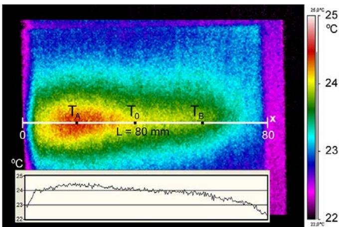
Fig. 6. Thermographic image of the surface of specimen 3 with the momentary temperature profile along the straight line representing the location of the adhesive layer axis
