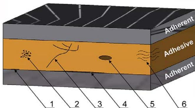
Fig. 1. Imperfections in adhesive lap joints; 1 – “kissing” bond, 2 – porosity, 3 – crack, 4 – delamination, 5 – cavity, 6 – poor cure
