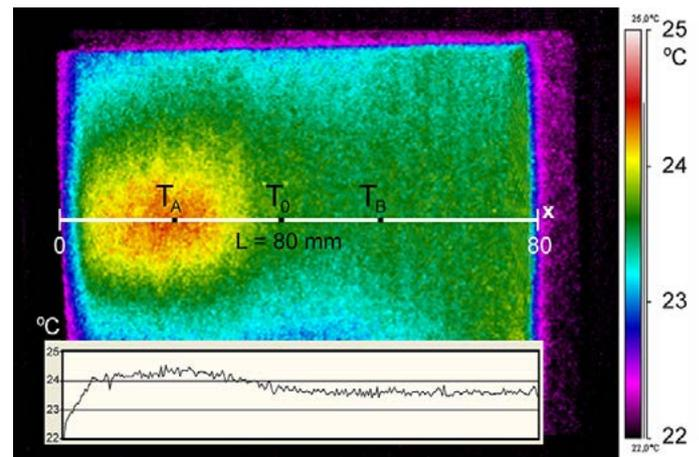
Fig. 5. Thermographic image of the surface of specimen 2 with the momentary temperature profile along the straight line representing the location of the adhesive layer axis
