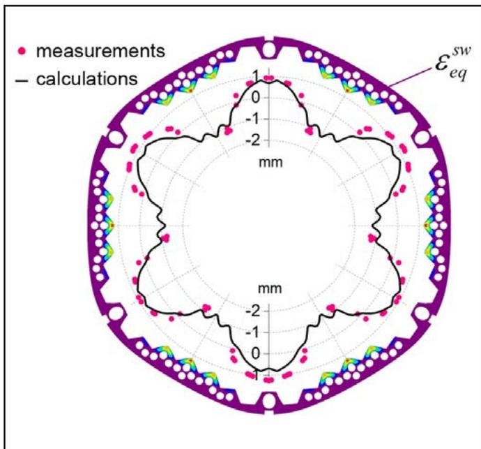
Fig. 4. Qualitative field of swelling, computational and experimental displacements of the internal surface of the enclosure of the active zone of the reactor in nuclear power plant JuUAES-2 during scheduled preventive maintenance after 30 years of operation, mm
