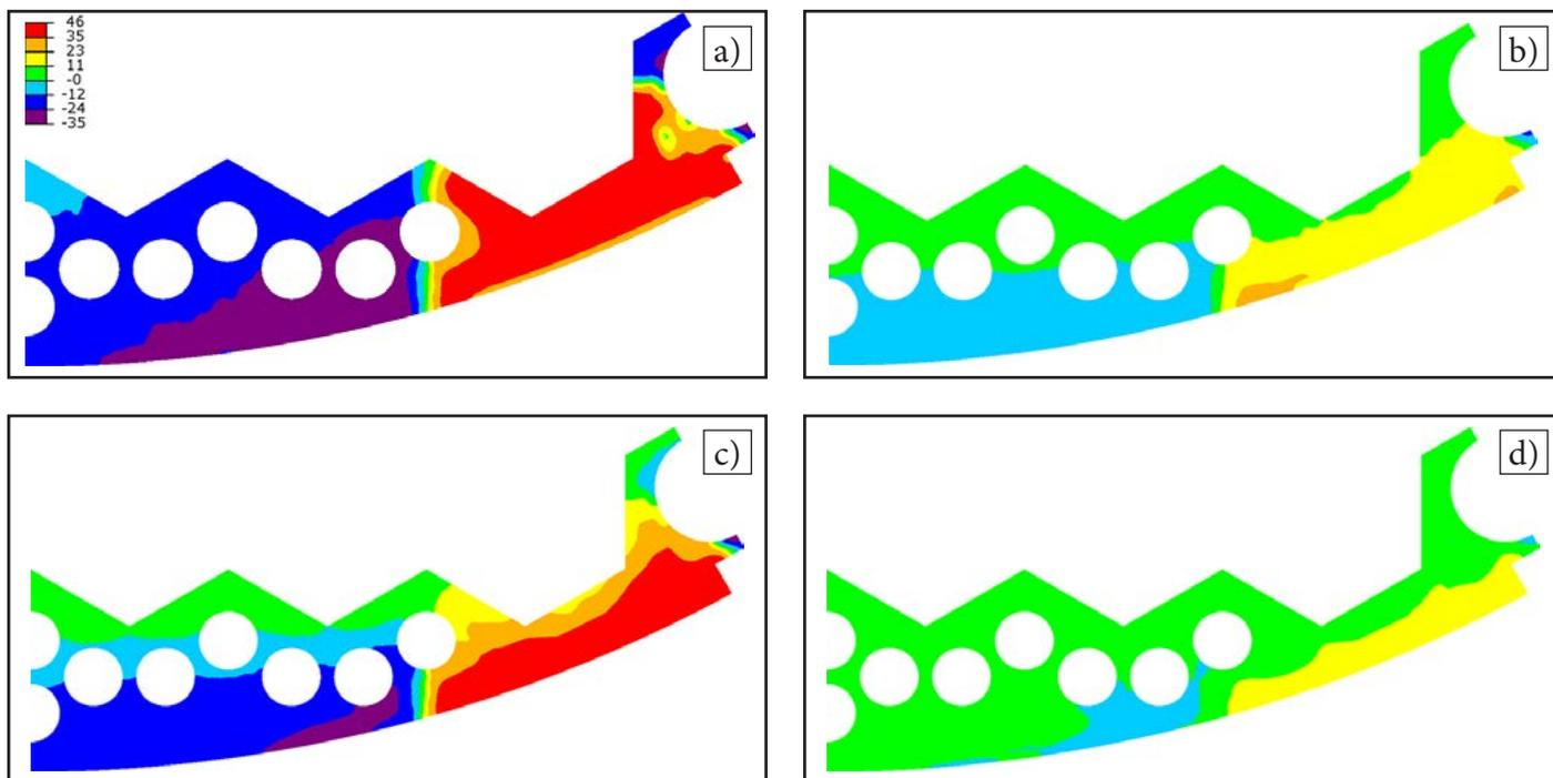
Fig. 8. Relaxation of welding internal stresses in the enclosure of the active zone of a WWER-1000 reactor: a) at the beginning of operation, b) after 20 years, c) after 40 years, d) after 60 years of operation
