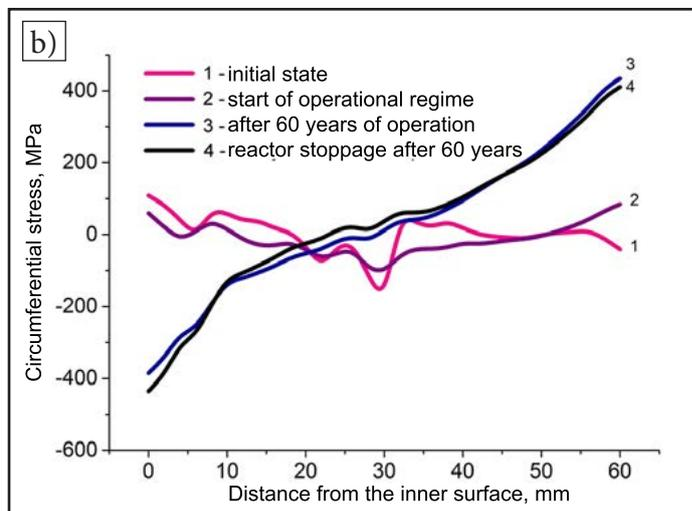
Fig. 5. Circumferential stresses across the thickness of the housing inside the reactor vessel taking into consideration the contact with the enclosure of the active zone: a) without welding internal stresses; b) including welding internal stresses
