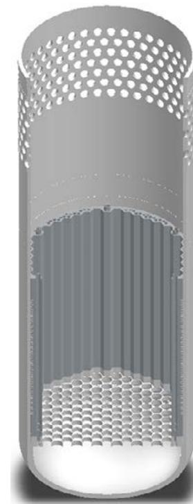
Fig. 1. Enclosure of the active zone and the chamber housing inside the WWER-1000 reactor vessel
