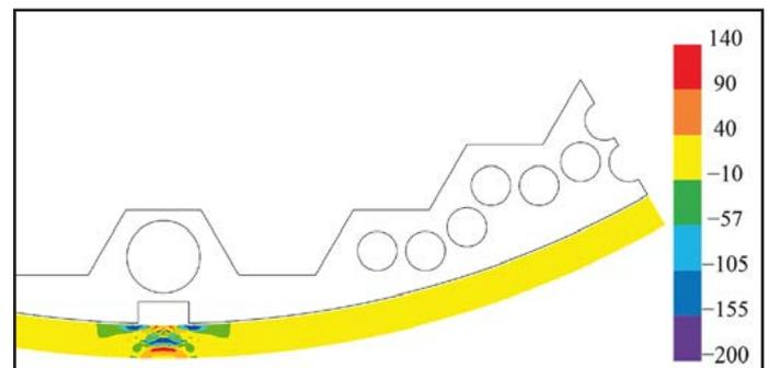
Fig. 2. Distribution of circumferential stresses in the weld zone of the housing of WWER-1000 reactor during production, MPa
