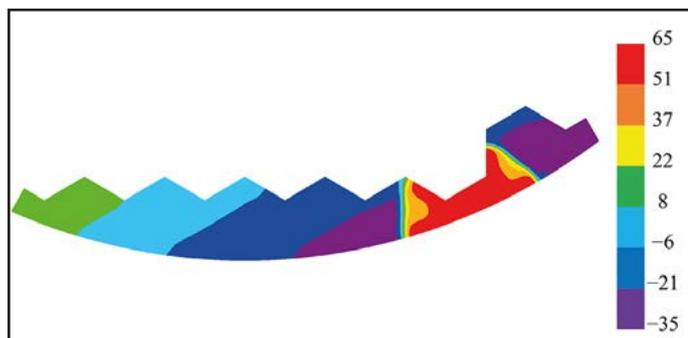
Fig. 3. Distribution of axial welding internal stresses in the enclosure of the active zone of a WWER-1000 reactor after heat treatment, MPa
