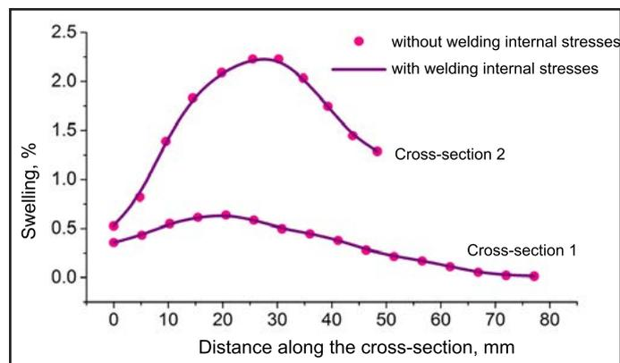
Fig. 6. Field of volumetric swelling strains in the active zone enclosure after 60 years of operation and the distribution of swelling in cross-sections 1 and 2, in problems taking and not taking into consideration welding internal stresses
