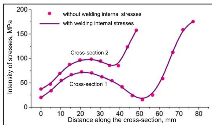
Fig. 7. Field of the intensity of stresses in the active zone enclosure after 60 years of operation and the distribution of stresses in cross-sections 1 and 2, in problems taking and not taking into consideration welding internal stresses
