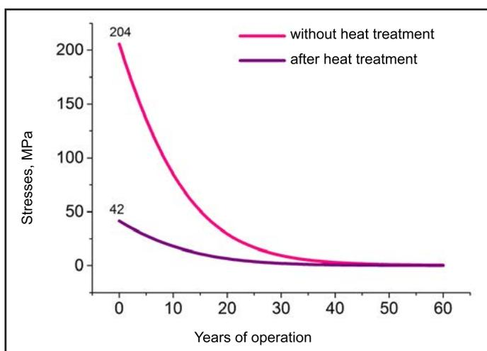
Fig. 9. Quantitative characteristics of the relaxation of welding internal stresses in the enclosure of the active zone of a WWER-1000 reactor during operation
