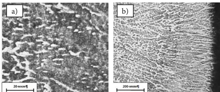
Fig. 5. Microstructure of the roller work surface metal surfaced using the Veltek-N545 flux-cored wire: a – mag. 1000x, b – mag. 100x
