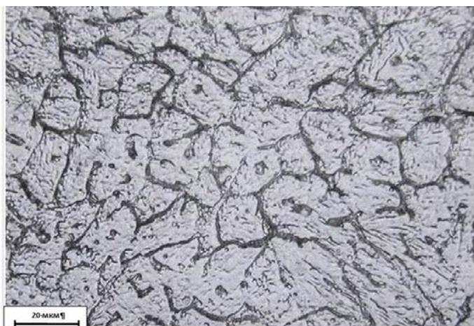
Fig. 6. Microstructure of the hardening layer metal subject to surfacing using the Veltek-N425 wire; mag. 1000x
