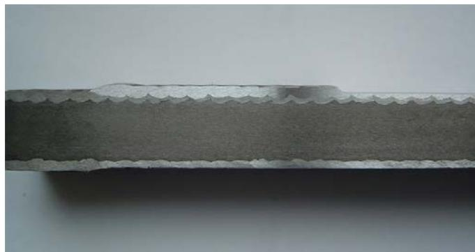
Fig. 7. Macrostructure of the surfaced plunger fragment
