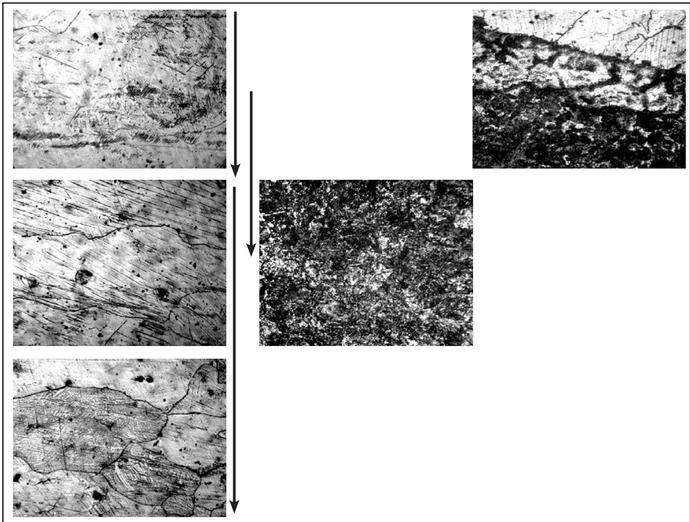
Fig. 4. Microstructures of layers surfaced using the Veltek-N285.01 flux-cored wire (from the surface to the base material). Mag. 550x
