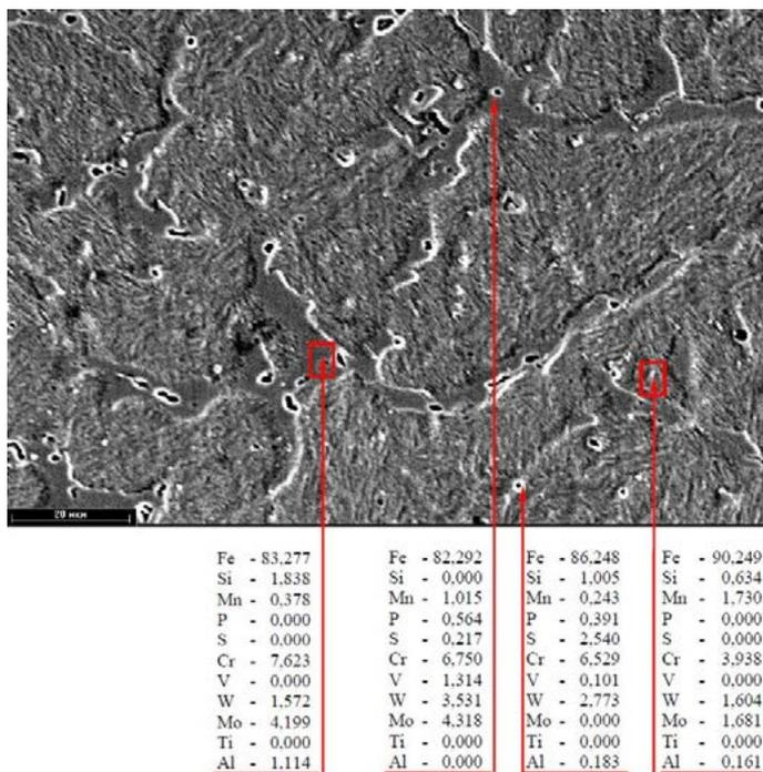
Fig. 2. Microstructure and the chemical composition of metal surfaced using the Veltek-N480NT wire
