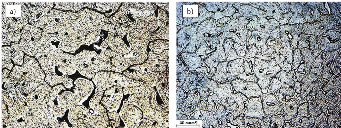
Fig. 1. Microstructure of metal surfaced using the wire: a – PP-Np-35W9H3SF, b – Veltek-N505RM; mag. 500x
