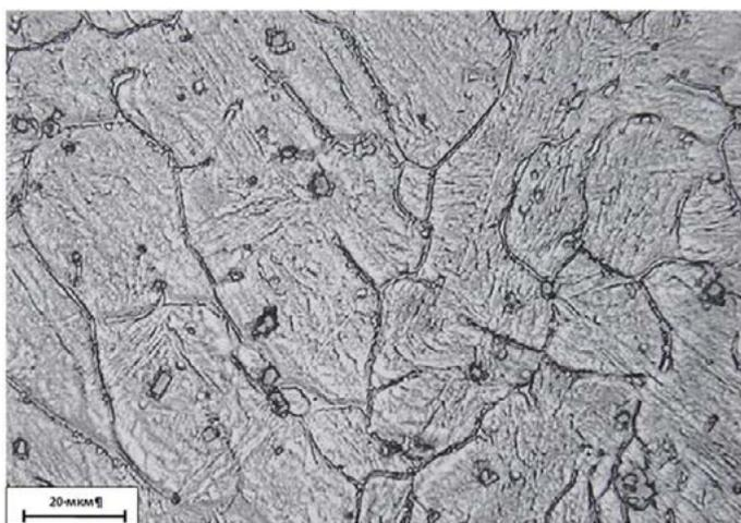
Fig. 3. Microstructure of the metal surfaced using the Veltek-N470 wire, volumetric content of  $\delta$  5.2%; hardness after surfacing 42÷46 HRC; mag. 1000x
