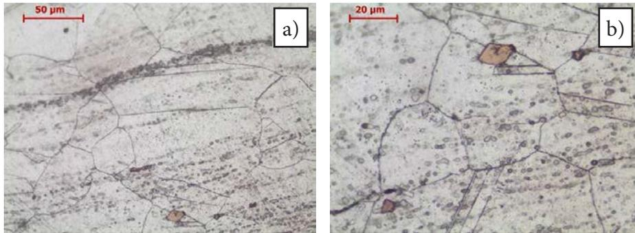
Fig. 3. Alloy 600; microstructure of the heat affected zone, visible grain growth – phase  $\gamma$  and carbide precipitates on the grain boundaries in within the grains
