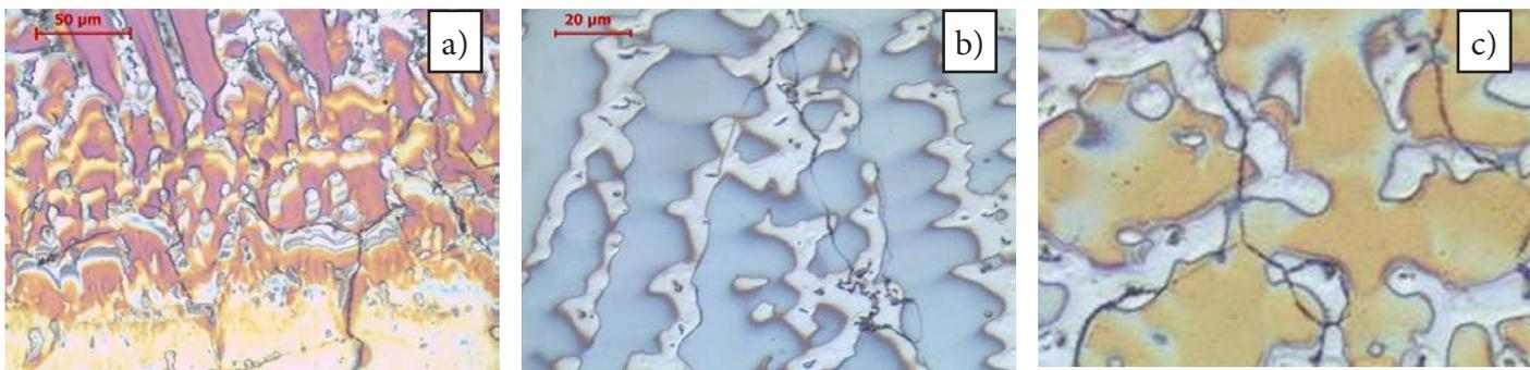
Fig. 8. Alloy 617; microstructure of the weld, visible grain growth; easily visible segregation of constituents in the interdendritic spaces with the formation of precipitates and other phases; dendrite cores having the structure of phase  $\gamma$
