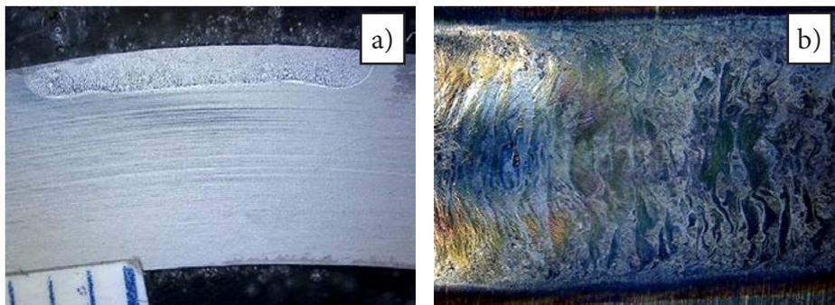
Fig. 5. Fusion in nickel alloy 617; current: 160 A: a) fusion macrostructure, b) weld face
