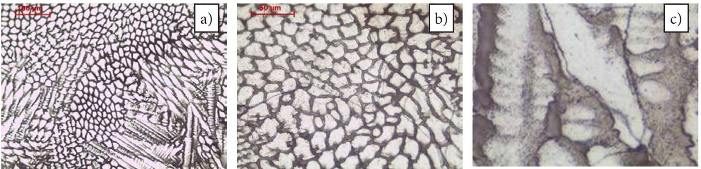
Fig. 4. Alloy 600; microstructure of the weld, cellular-dendritic structure; dendrite cores having the structure of phase  $\gamma$
