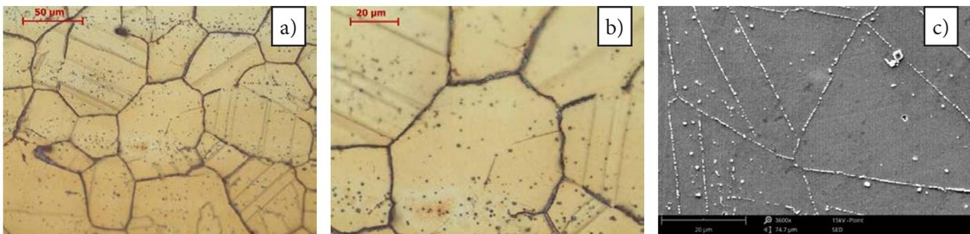
Fig. 6. Alloy 617; microstructure in the base material area (as-delivered state): a-b) light microscopy, c) SEM; visible decorated twin boundaries (annealing twins); structure of phase  $\gamma$  with carbide precipitates forming the lattice on the grain boundaries in within the grains
