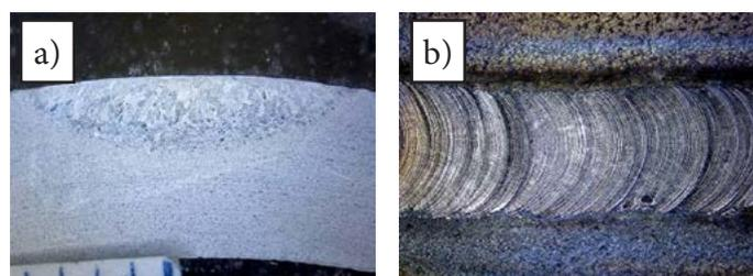
Fig. 1. Fusion in nickel alloy 600; current: 160 A: a) fusion macrostructure, b) weld face
