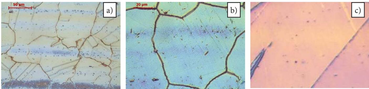
Fig. 7. Alloy 617; microstructure in the heat affected zone, visible grain growth; visible banding and twin boundaries (annealing twins); visible lattice of precipitates on the grain boundaries
