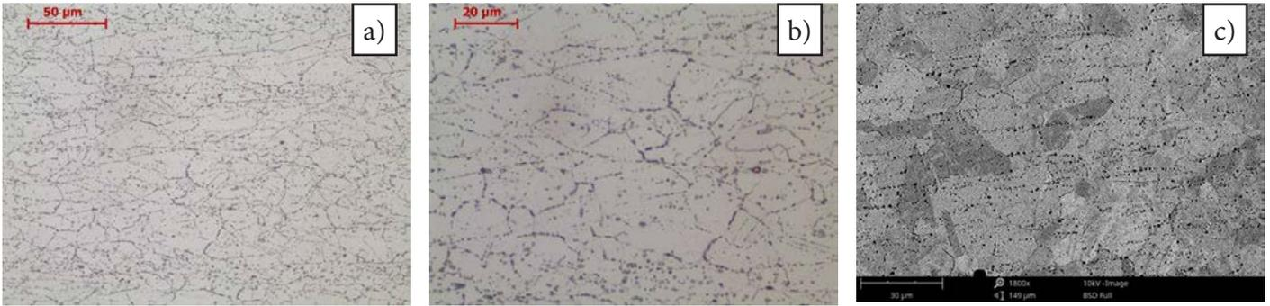
Fig. 2. Alloy 600; microstructure in the base material area (as-delivered state): a-b) light microscopy, c) SEM; structure of phase  $\gamma$  with carbide precipitates on the grain boundaries in within the grains
