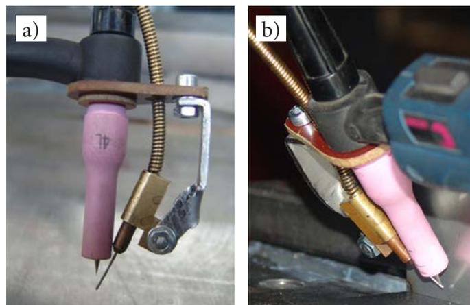
Fig. 6. Modernised wire feeder fixed on the TIG welding torch of the LORCH V40 AC/DC welding machine: a) main view; b) position during the welding of a T-joint
