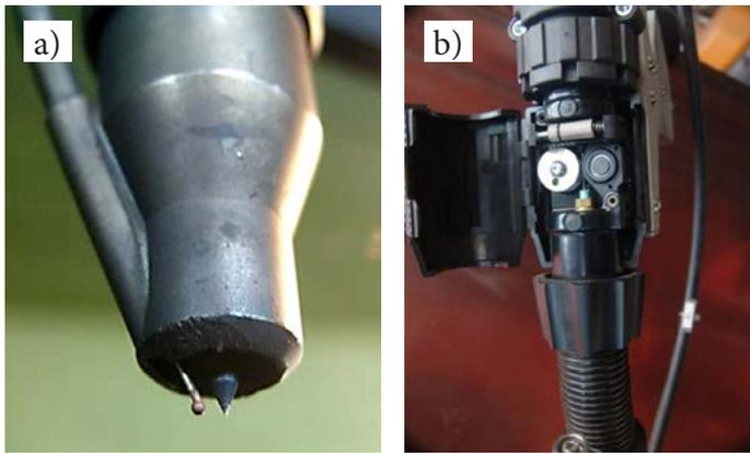
Fig. 2. View: a) gas nozzle of the TOPTIG welding torch with the wire feeding conduit; b) wire feeder in the upper part of the TOPTIG welding torch
