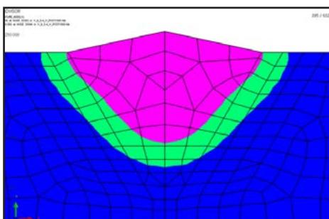
Fig. 5. Macrostructure of the butt joint bead made of S355 steel, the shape of the liquid metal pool corresponding to the macrostructure and the HAZ area during a numerical simulation
