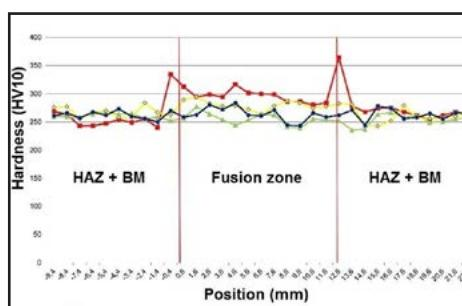
Fig. 4. Results of hardness and strains measurements of a tested joint
