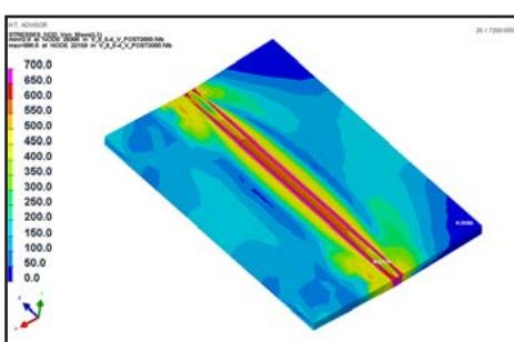
Fig. 6. Distribution of post-weld joint strains (left) and stresses (right)
