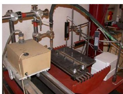
Fig. 3. Welding station used in tests and exemplary thermal cycles recorded when welding joints made of S355 steel
