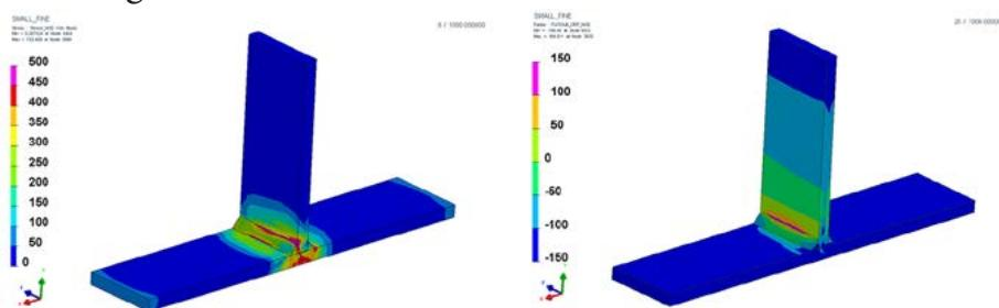
Fig. 2. Distribution of post-weld stresses and the result of high-cycle load analysis according to the Van Dang criterion
