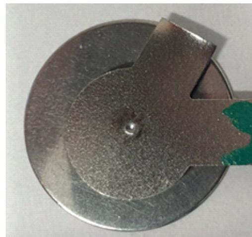
Fig. 1. Element subjected to laser beam welding
