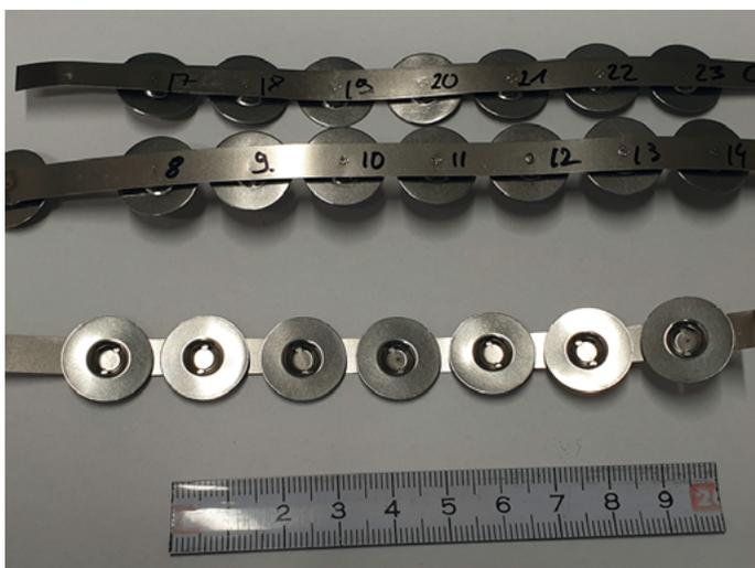
Fig. 9. Laser beam welded joints
