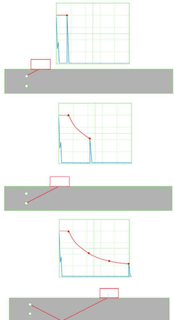
Fig. 5. Plotting of the comparative line using the lines of pass-through holes
