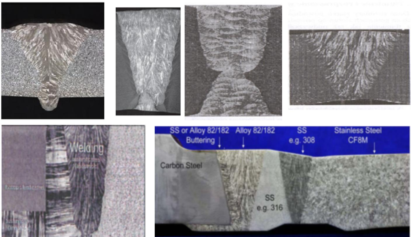
Fig. 1. Weld in the similar joint (a), coarse-grained structure (b) and dissimilar material weld (c)
