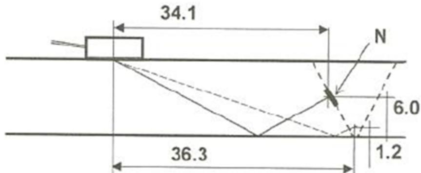
Fig. 2. Change of the diffraction angle of ultrasonic beam insertion
