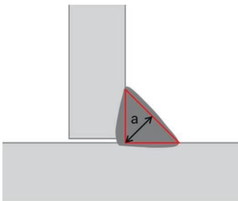
Fig. 1. T-joint with the fillet weld and dimension  $a$
