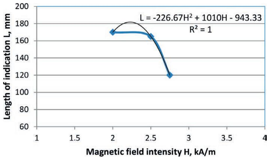
Fig. 16. Correlation between lengths of indications and values of magnetic field intensity in relation to the area of highest sensitivity
