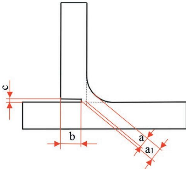
Fig. 3. Schematic diagram of the standard specimen, where  $a$  – fillet weld dimension,  $a_1$  – distance between the weld face and the bottom of the incision,  $b$  – incision depth and  $c$  – incision width
