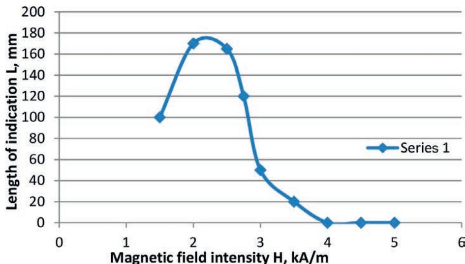
Fig. 15. Correlation between lengths of indications and values of magnetic field intensity
