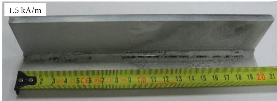
Fig. 7. Indications obtained in relation to a magnetic field intensity of 1.5 kA/m
