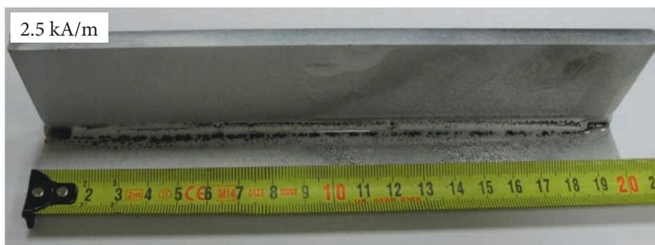
Fig. 9. Indications obtained in relation to a magnetic field intensity of 2.5 kA/m
