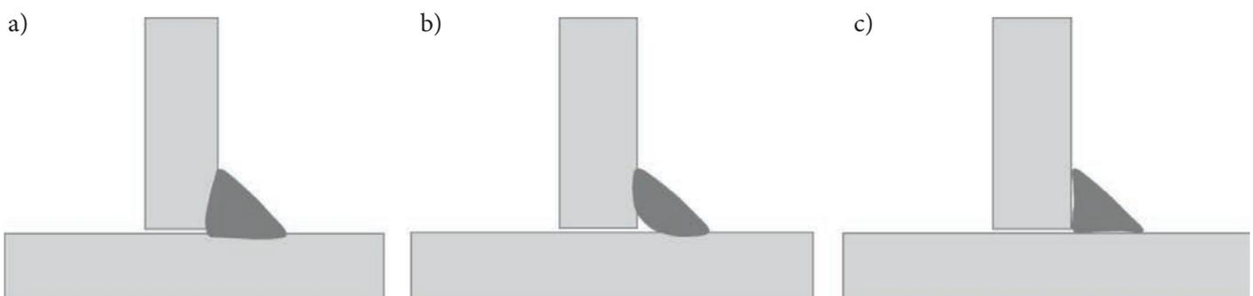
Fig. 2. T-joint with the fillet weld: a) proper penetration, b) lack of penetration and c) incomplete fusion
