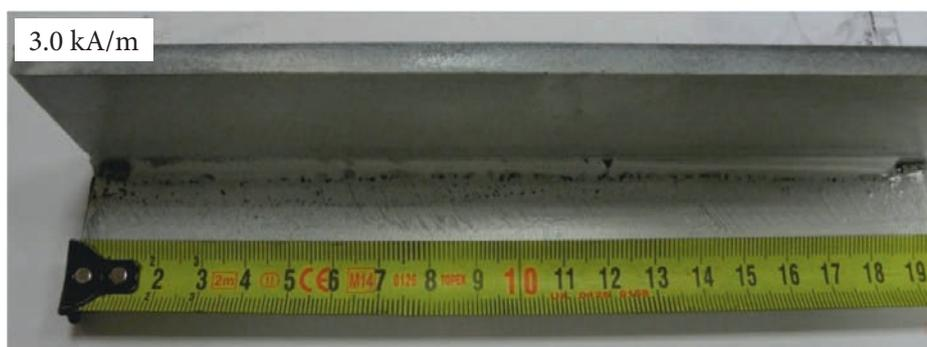
Fig. 10. Indications obtained in relation to a magnetic field intensity of 3.0 kA/m
