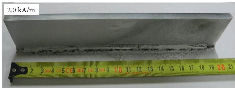
Fig. 8. Indications obtained in relation to a magnetic field intensity of 2.0 kA/m
