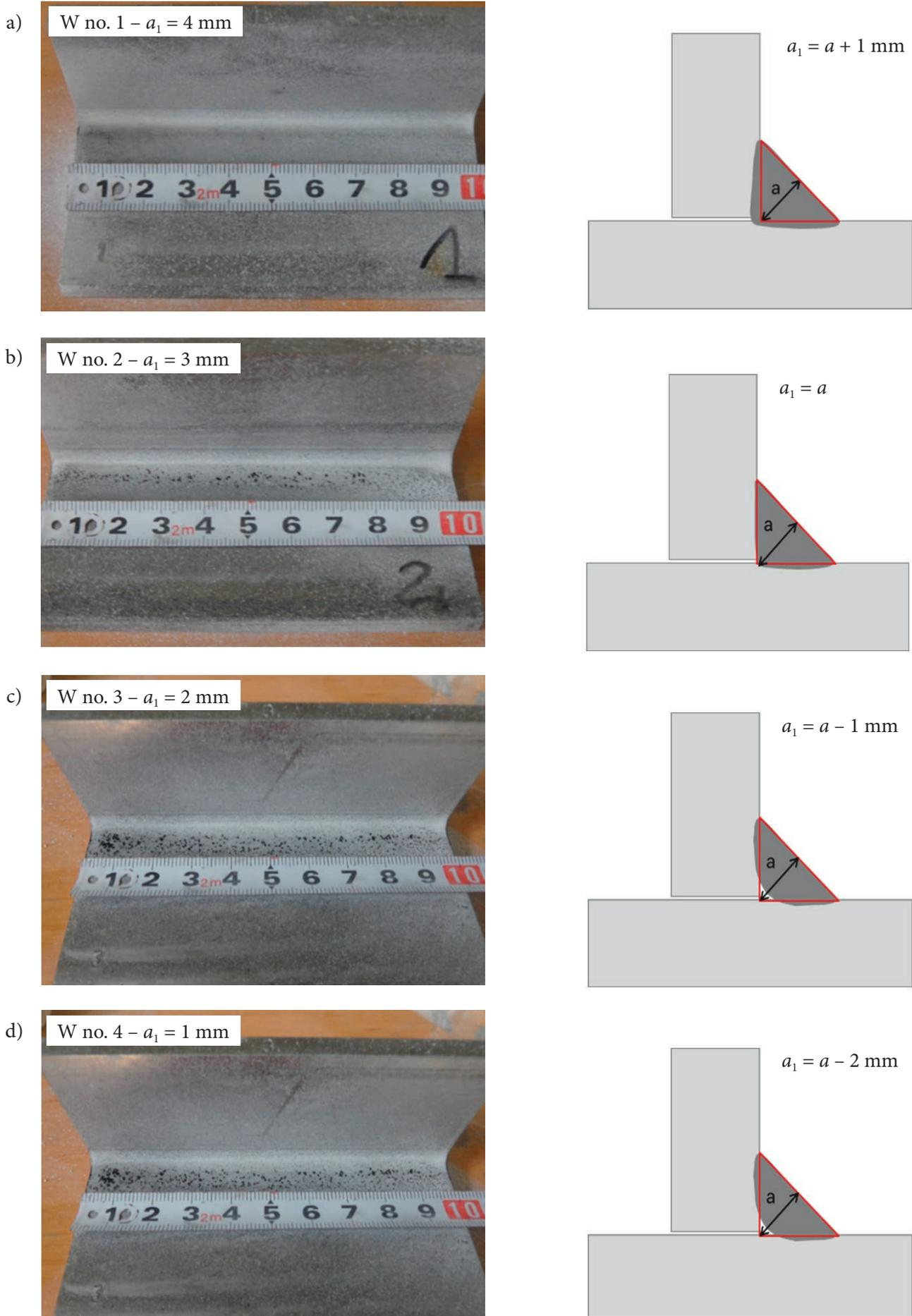
Fig. 4. Indications revealed in standard specimens nos. 1 through 4 along with the illustration of the simulated discontinuity in the T-joints: a) simulation at the ultimate detection sensitivity in the magnetic particle testing method, b) simulation of proper penetration having a depth of 1 mm, c) simulation at the verge of penetration and d) simulation of the significant lack of penetration
