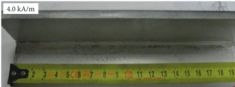
Fig. 12. Indications obtained in relation to a magnetic field intensity of 4.0 kA/m
