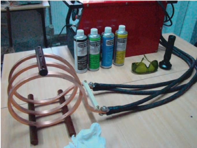
Fig. 5. Magnetic particle testing station with the electromagnetic coil
