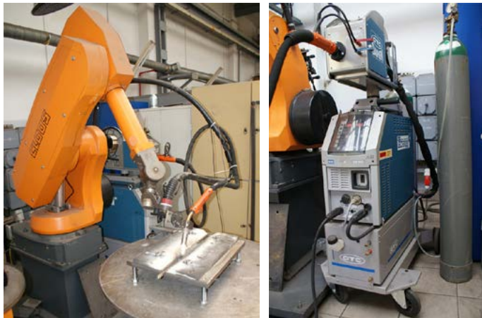
Fig. 4. Test rig for braze welding (left), a DW-300+ welding device by DAIHEN (right)
