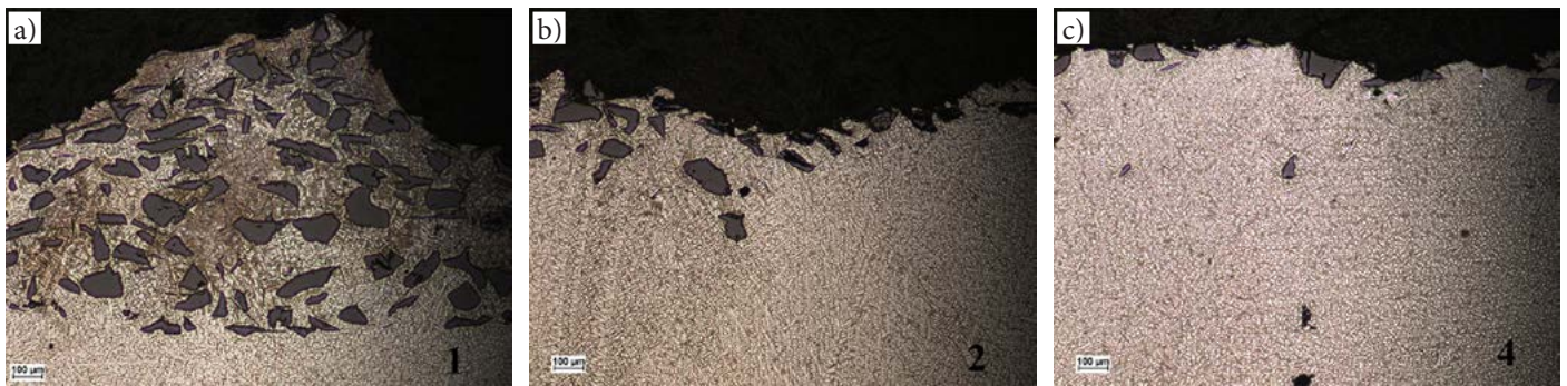
Fig. 11. Microstructure of the cross-section of surface alloyed runs made with a HPDDL on an AlSiCu4MgMn aluminium alloy base. Surface alloying parameters: the laser beam power of 2000 W, the surface alloying rate of 0.25 m/min, the powder feeding rate of: a) 1.5 g/min; b) 1 g/min; c) 0.5 g/min. Note: test piece designations as in Table 3
