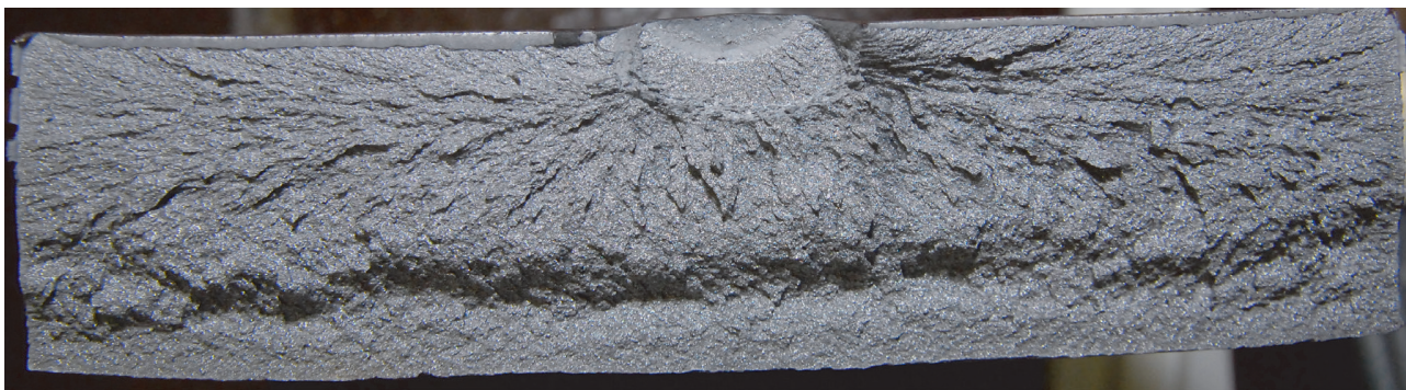
Fig. 8. Cross-section of specimen no. 1/60 containing the bend-triggered fracture
