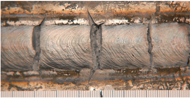
Fig. 4. Cracks in the overlay weld at the initial stage of bending
