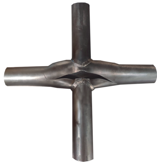
Fig. 10. Welded joint after the tensile test
