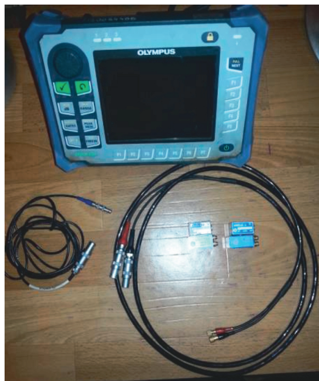
Fig. 7. Ultrasonic flaw detector (EPOCH 650) along with signal cables and ultrasonic transducers
