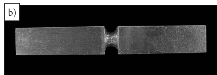
Fig. 4. Specimens with the simulated HAZ area used in the toughness and hardness (a) as well as tensile strength (b) tests
