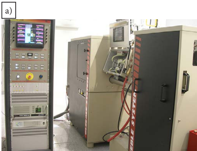
Fig. 3. Gleeble 3500 simulator (a) and the exemplary curve of specimen heating and cooling cycle (b)
