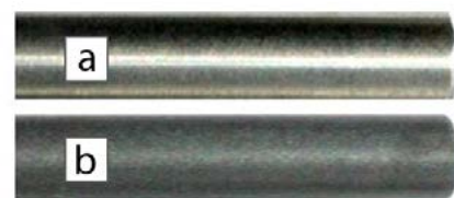
Figure 8. General view of fragments of zirconium shells without coating (a) and with coating (b) on silicon carbide base
