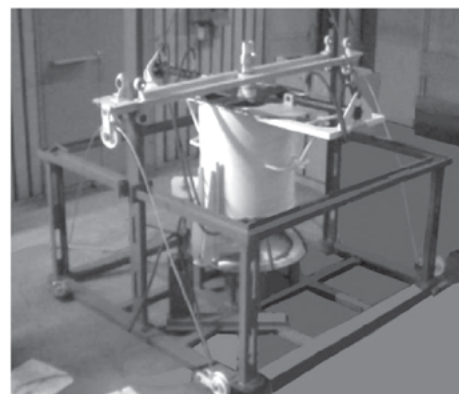
Figure 20. Module for joining the damaged pipes of wells
