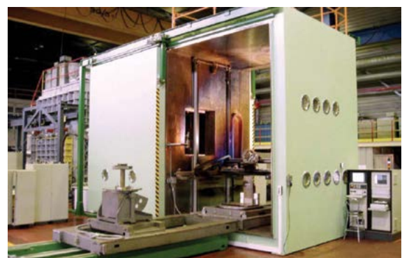
Figure 6. EBW equipment manufactured at the E.O. Paton Electric Welding Institute
