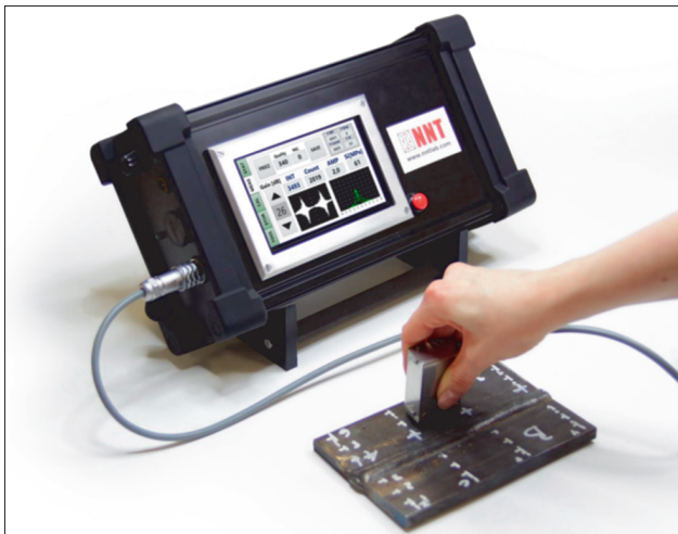
Fig. 5. Fifth generation stress meter MagStress5C [9]
