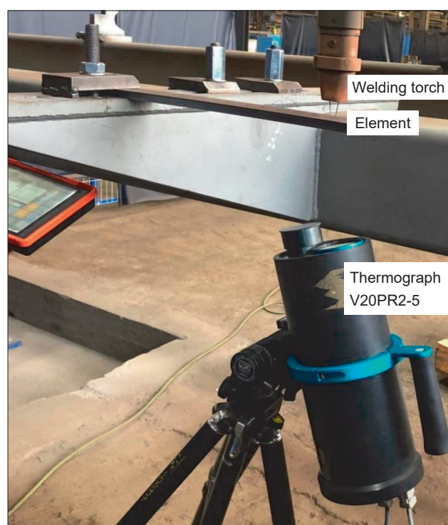
Fig. 1. Non-contact measurement of temperature during the MAG STANDARD and MAG TANDEM processes
