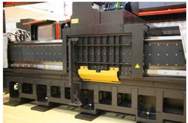
Fig. 6. Linear drive placed on the side (good protection against impurities) of Amada FOL 3015 NT laser cutter [6]
