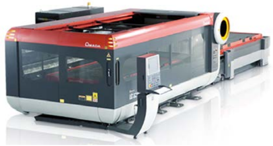
Fig. 5. 2D laser cutter series LC-F1 NT manufactured by Amada, provided with linear drives [6]
