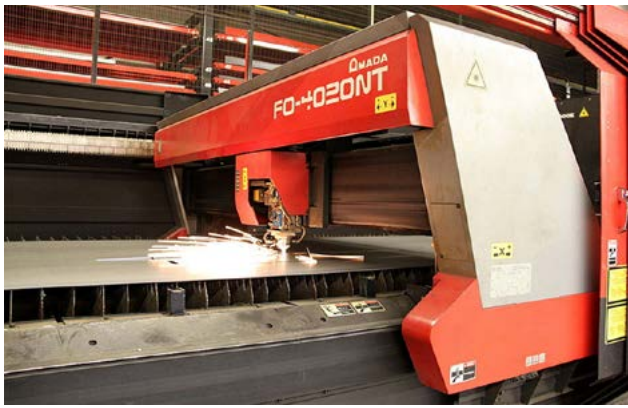
Fig. 1. Laser cutter with a CO 2 laser and a "flying optics" system [6]
