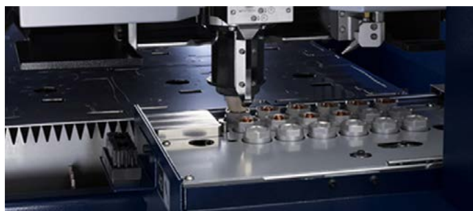
Fig. 15. Pallet with exchangeable nozzles in a modern cutter produced by Trumpf [4].
