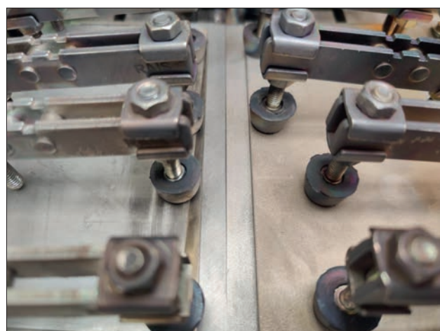
Fig. 6. Positioning grip fixed on the work table of the electron beam welding machine
