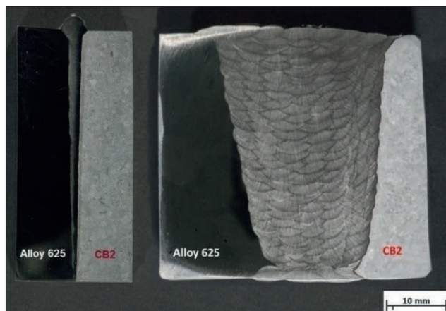
Fig. 3. Electron beam welded joint (left) and the joint obtained using the MMAW process (right) [21]
