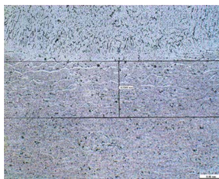
Fig. 3. Microstructure of the overlay weld made with 45% EN ratio; HAZ width: 0.151 mm, mag. 200x, etching with Keller's reagent
