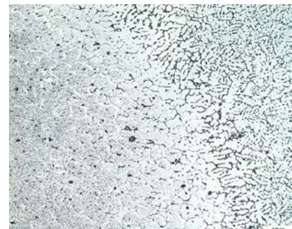
Fig. 12. Microstructure of the joint made of 1 mm thick EN AW 6082 alloy, the view in the fusion area (on the right – the weld, on the left – the base metal), etching with Keller's reagent, mag. 200x
