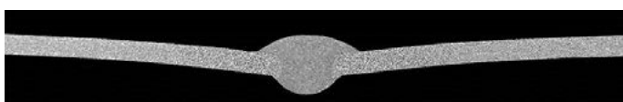
Fig. 10. Macrostructure of the butt joint made of 1 mm thick EN AW 5754 alloy sheets, mag. 4x; welding parameters: I=20 A; U=18.0 V; V_{sp}=55 cm/min., EN=60\% , frequency 3 Hz
