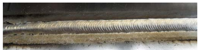
Fig. 15. View of the weld face in the T-joint with the fillet weld made of 3 mm thick EN AW 5754 alloy sheets using the AC Wave Pulse variant
