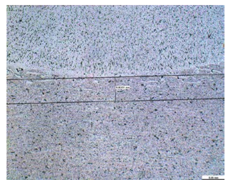
Fig. 4. Microstructure of the overlay weld made with 80% EN ratio; HAZ width: 0.0643 mm, mag. 200x, etching with Keller's reagent
