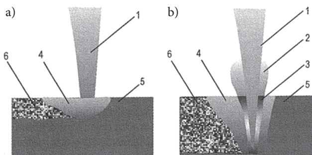
Fig. 2. Laser beam welding process: a) melt-in technique and b) key-hole technique: 1 – laser beam, 2 – plasma cloud, 3 – capillary (key-hole), 4 – molten metal pool, 5 – base material and 6 – molten material [9]
