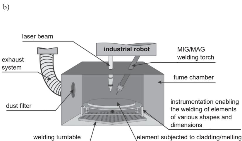
Fig. 3. Experimental station for testing the emission of pollutants during laser beam welding: a) main view and b) schematic diagram [7, 10]
