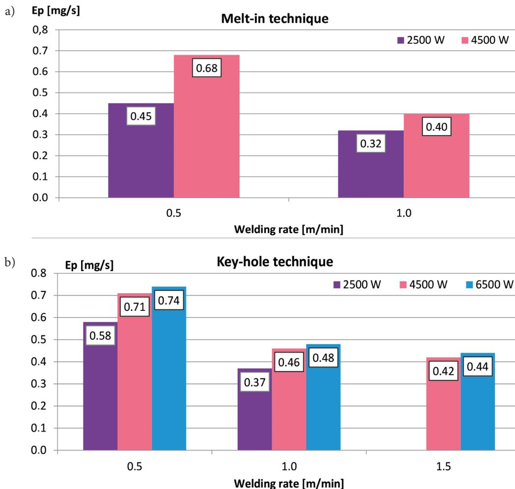
Fig. 6. Effect of the welding rate on the emission of total dust in time during the laser beam welding of steel 1.4301: a) melt-in technique and b) key-hole technique [7]
