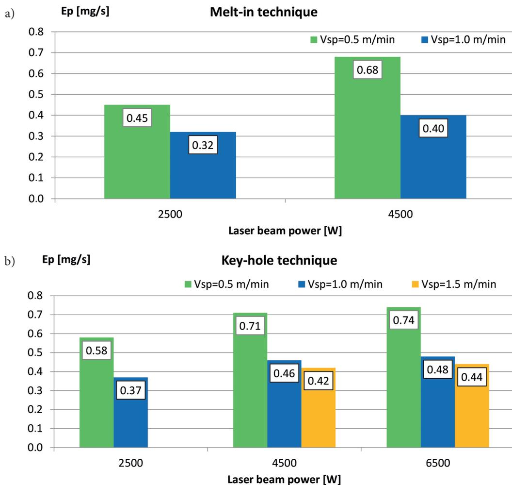
Fig. 5. Effect of laser beam power on the emission of total dust in time during the laser beam welding of steel 1.4301: a) melt-in technique and b) key-hole technique [7]
