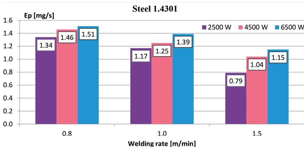
Fig. 9. Effect of the welding rate on the emission of total dust in time during the hybrid welding (HLAW) of steel 1.4301 [7]
