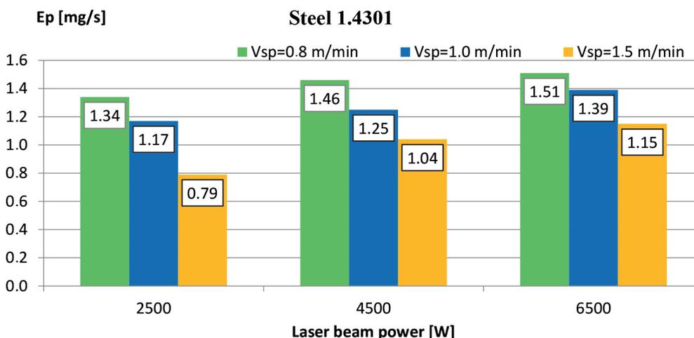
Fig. 7. Effect of laser beam power on the emission of total dust in time during the hybrid welding (HLAW) of steel 1.4301 [7]
