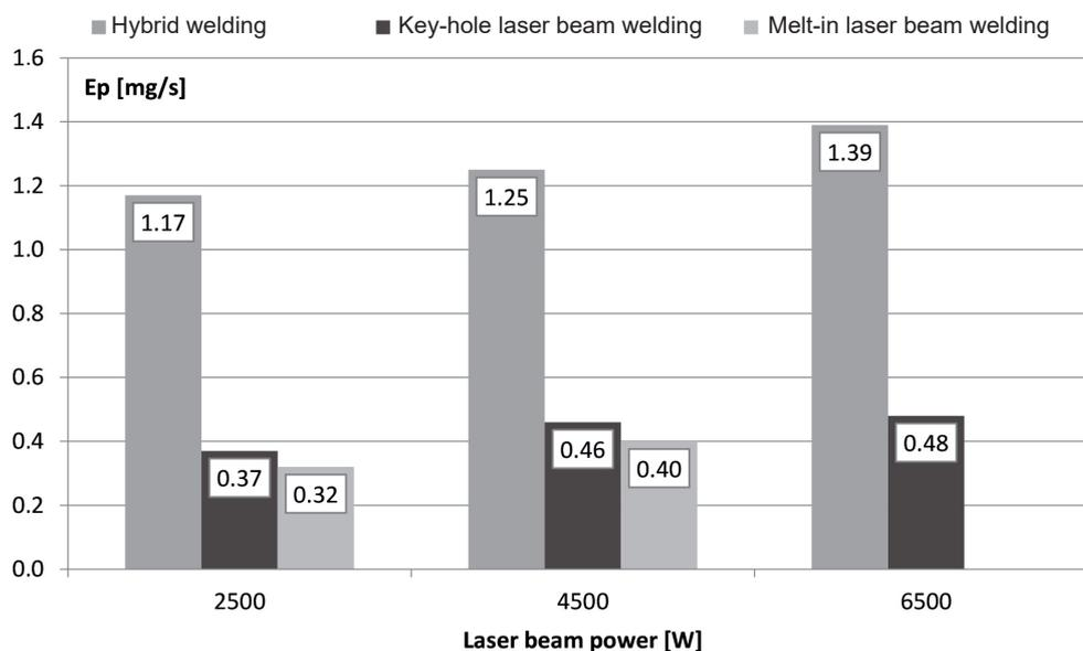
Fig. 10. Comparison of indicators concerning the emission of total dust in time in relation to the laser beam welding and hybrid welding of steel 1.4301 [7]
