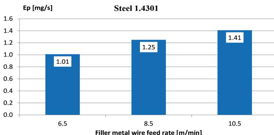
Fig. 8. Effect of the filler metal wire feed rate on the emission of total dust in time during the hybrid welding (HLAW) of steel 1.4301 [7]
