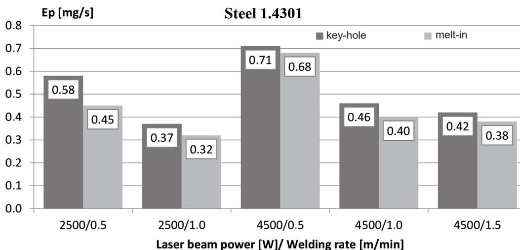
Fig. 4. Effect of a welding technique on the emission of welding fume in time during the laser beam welding of steel 1.4301 [7]
