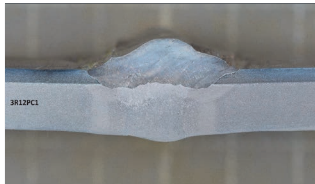
Fig. 6. Macrostructure of the overlay weld of Sanicro 3R12/4L7; external layer was obtained using the cladding process and rutile electrode Cromarod 309MoL
