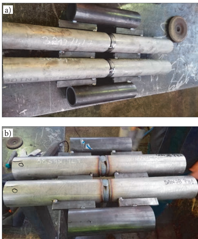
Fig. 4. Weld face view of the joints obtained using the conventional welding process: a) tube 3R12/4L7 and b) tube Sanicro 38/4L7
