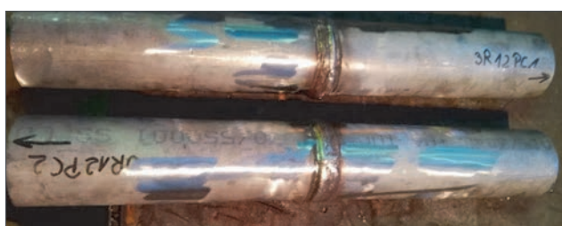
Fig. 5. Weld face view of the joint after the cladding process - tube 3R12/4L7
