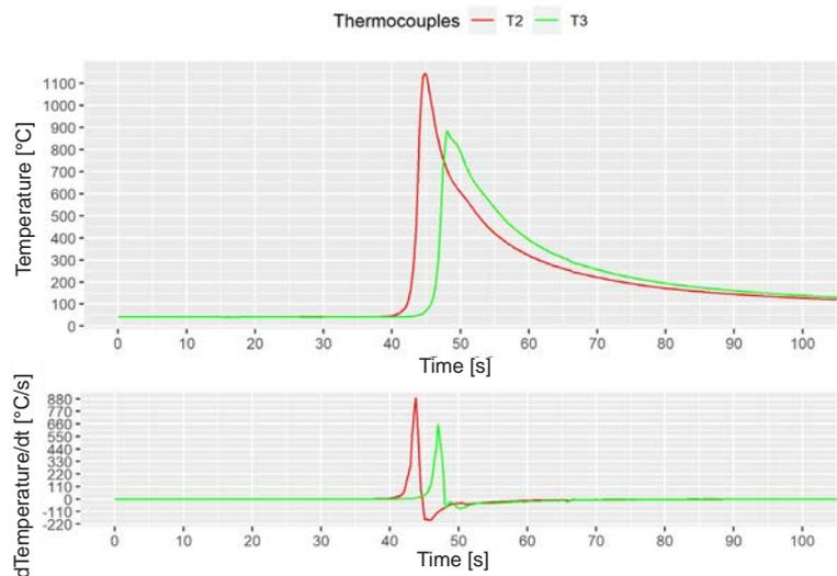
Fig. 3. Joint no. I – welding thermal cycle during hand-held laser welding (distance between the thermocouples and the weld axis: 2 mm, thermocouples T2 and T3) and the rate of temperature changes
