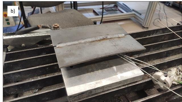
Fig. 2. Station for TIG welding along with necessary measurement equipment
