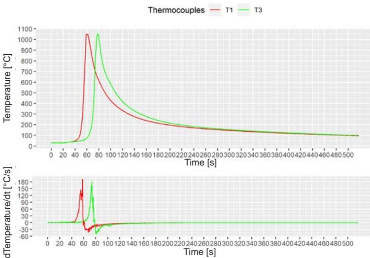
Fig. 8. Joint no. III – welding thermal cycle during hand-held laser welding (distance between the thermocouples and the weld axis: 4 mm, thermocouples T1 and T3) and the rate of temperature changes
