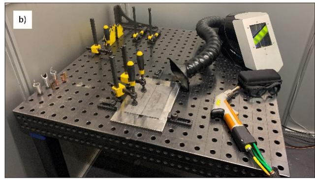
Fig. 1. Hand-held laser beam welding station along with necessary measurement equipment
