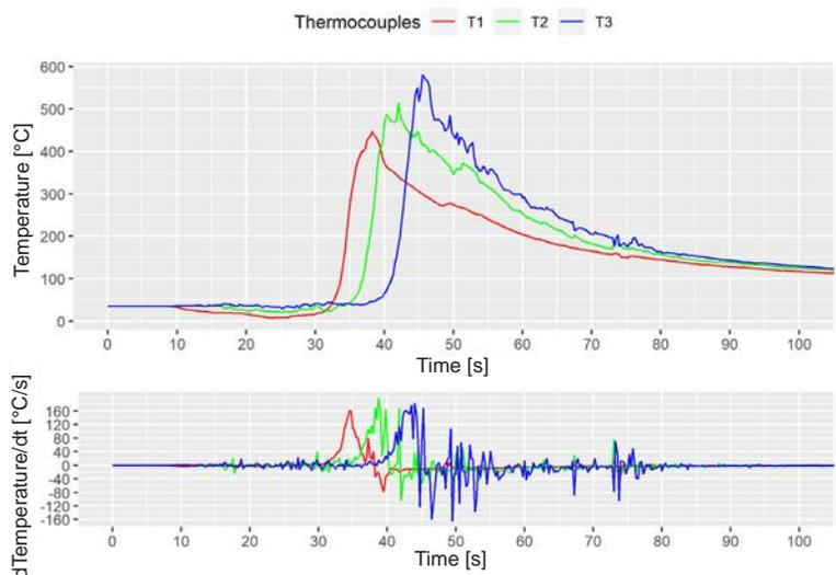
Fig. 4. Joint no. I – welding thermal cycle during hand-held laser welding (distance between the thermocouples and the weld axis: 4 mm, thermocouples T1, T2 and T3) and the rate of temperature changes
