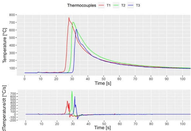
Fig. 5. Joint no. II – welding thermal cycle during hand-held laser welding (distance between the thermocouples and the weld axis: 2 mm, thermocouples T1, T2 and T3) and the rate of temperature changes
