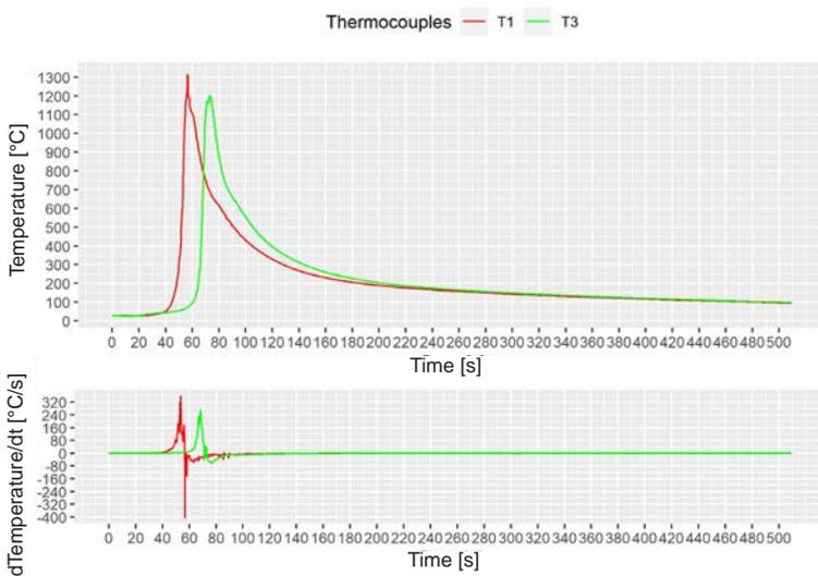
Fig. 7. Joint no. III – welding thermal cycle during hand-held laser welding (distance between the thermocouples and the weld axis: 2 mm thermocouples T1 and T3) and the rate of temperature changes
