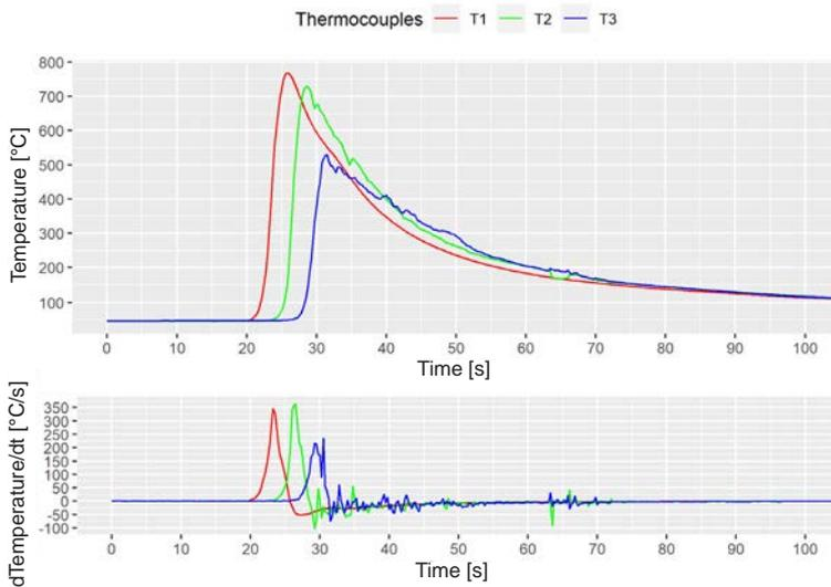
Fig. 6. Joint no. II – welding thermal cycle during hand-held laser welding (distance between the thermocouples and the weld axis: 4 mm, thermocouples T1, T2 and T3) and the rate of temperature changes
