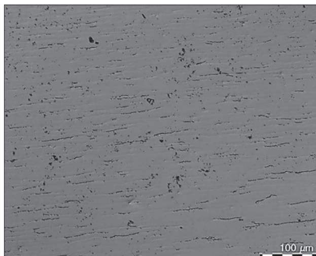
Fig. 1. Microstructure of the base material, i.e. steel X5CrNi18-10
