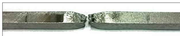
Fig. 7. Specimen after the static tensile test
