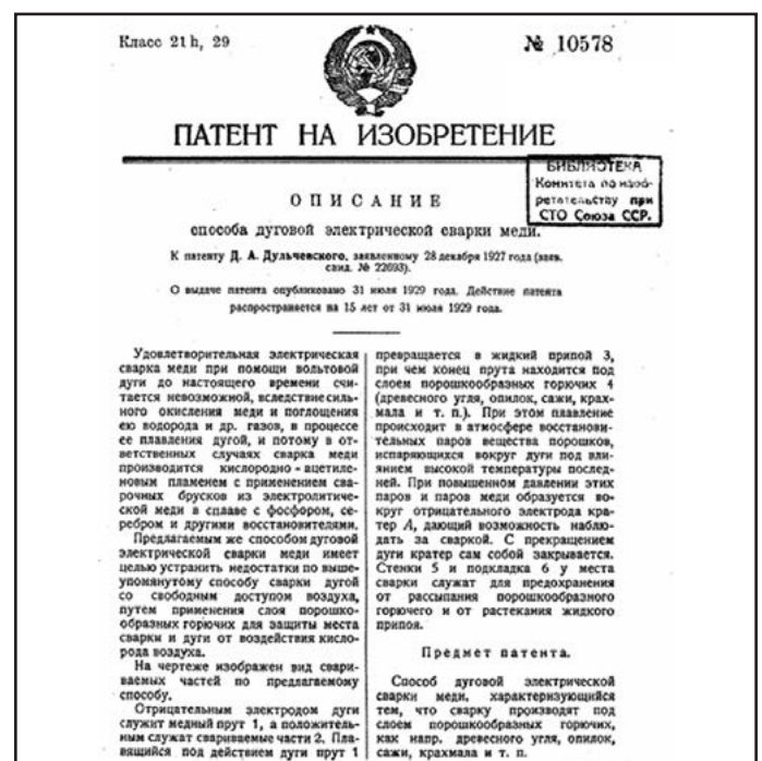
Fig. 3. USSR patent no. 10578 for arc welding of copper, page 1 of the description [9]
