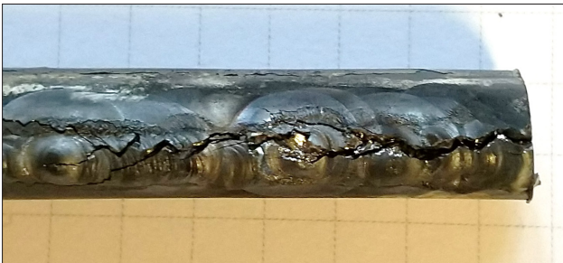
Fig. 10. Crack in the weld of test joint 3A after the crush test
