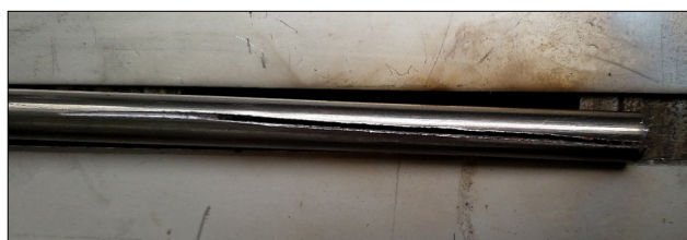
Fig. 5. Tube (Ø10×1 mm) after square butt weld preparation
