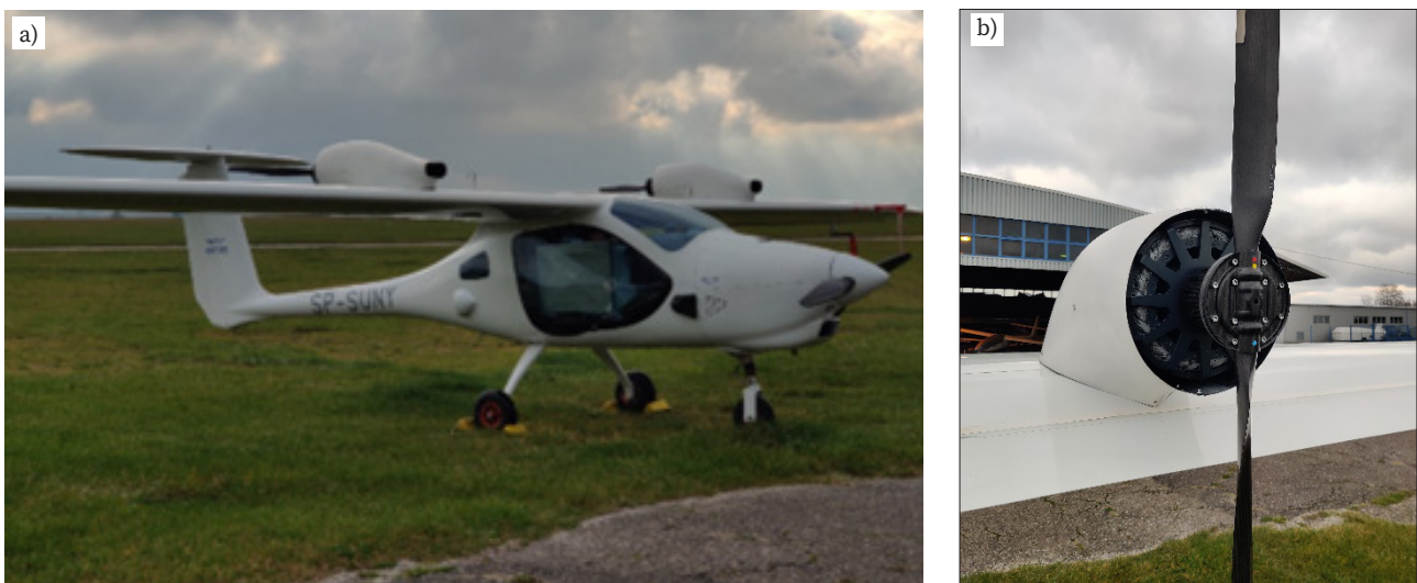
Fig. 7. a) Prototype hybrid aircraft and b) LEMoK 300 motor installed in a nacelle on the aircraft wing
