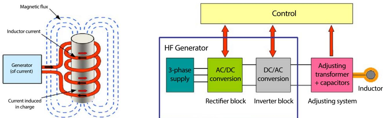
Fig. 1. Induction heating method and heating device block diagram
