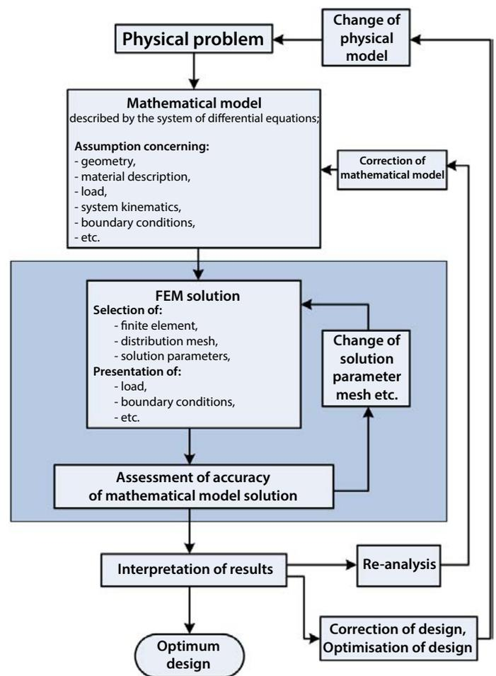
Fig. 5. Method used for FEM-based computer modelling
