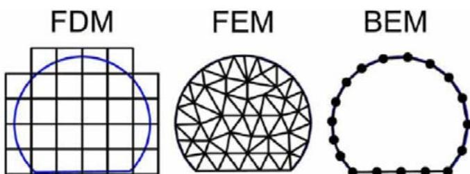
Fig. 4. Discretisation manner depending on simulation method
