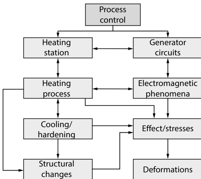
Fig. 6. Structure of induction heating process model
