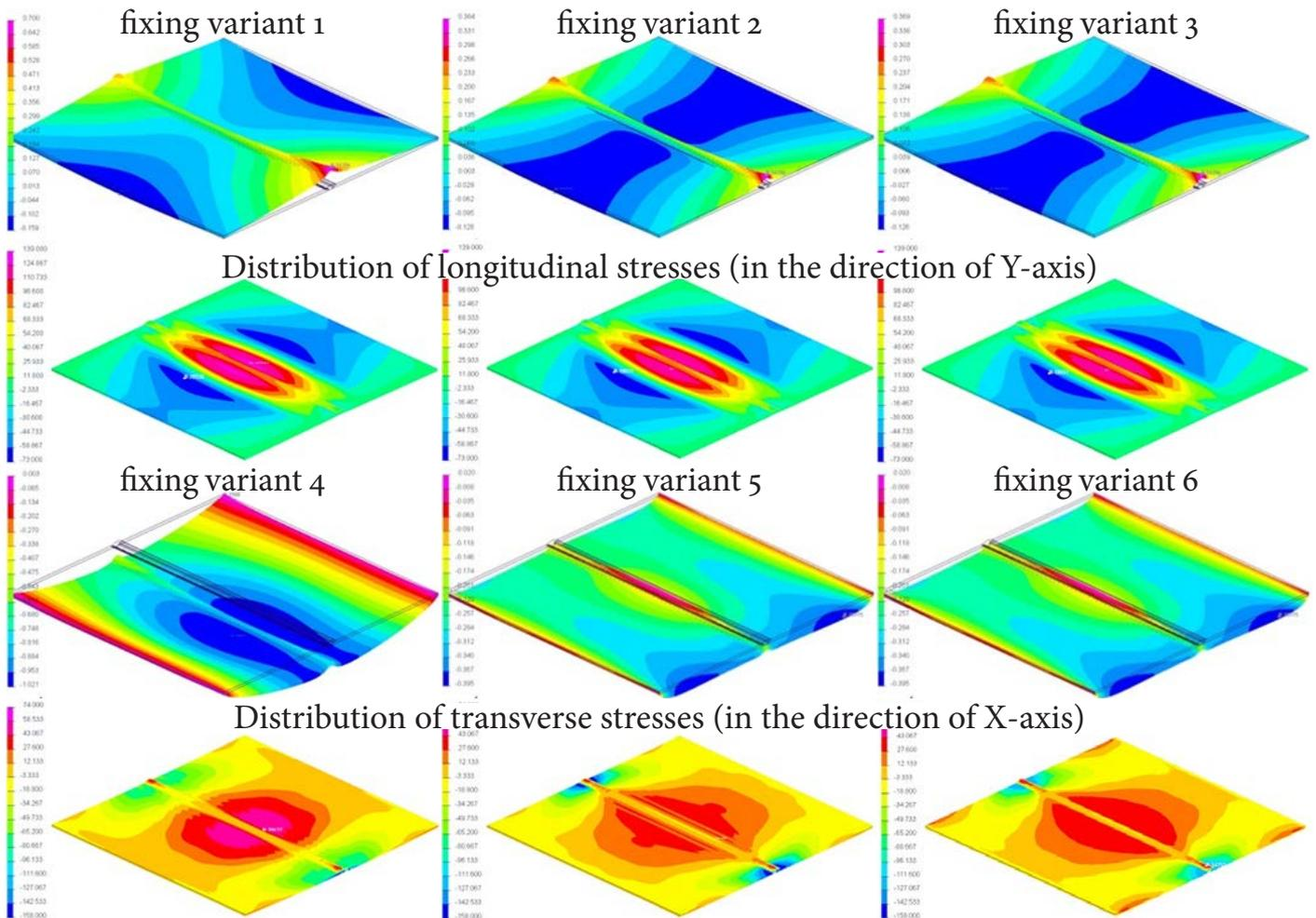
Fig. 11. Strains in the direction of Z-axis for various manners of element fixing during welding and corresponding distributions of longitudinal and transverse stresses, Table 2
