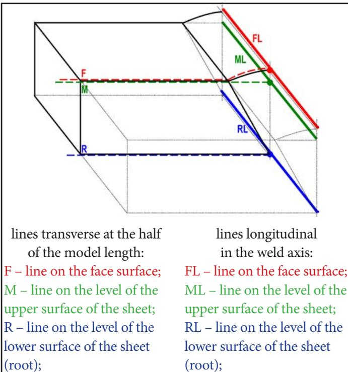
Fig. 7. Position of lines for determining the level of stresses in the model analysed
