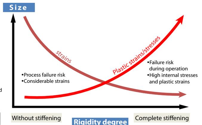
Fig. 2. Opposing effect of structural rigidity on plastic strains and internal stresses [14]
