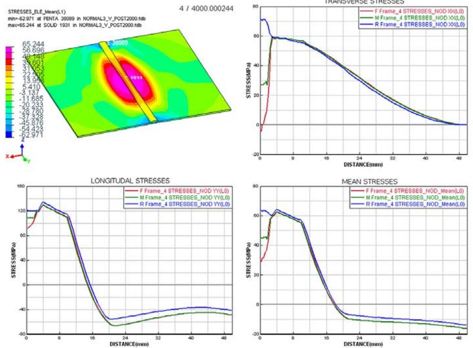
Fig. 8. Distribution of stresses on the cross-section at the half of the joint length – sheet fixing manner: variant no. 1 – Table 3
