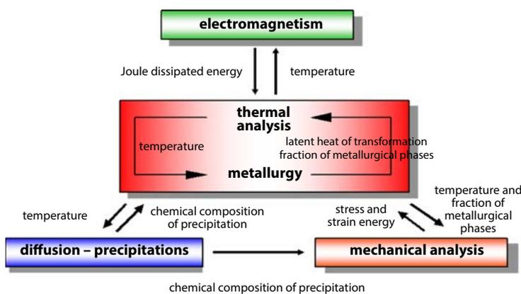
Fig. 1. SYSWELD structure [14]
