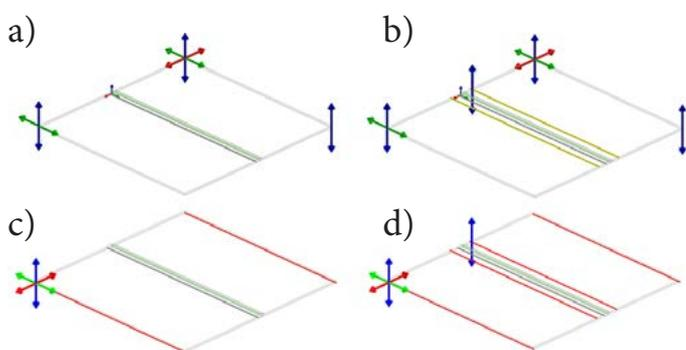
Fig. 5. Sheet fixing variants during analysis – ‘rigid’ fixing (arrows designate taking away the freedom degrees of a point in the indicated direction, in Figures C and D – all the points on the red line and in Figure B along the yellow line)
