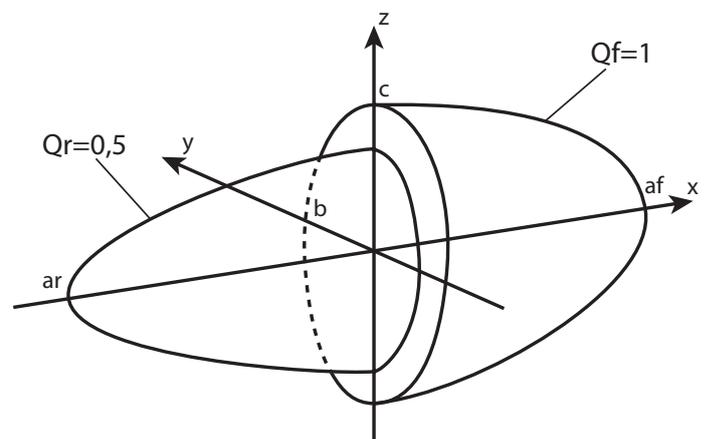
Fig. 3. Double-ellipsoidal heat source model (the Goldak model) [14]
