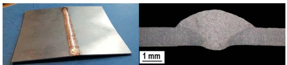
Fig. 10. Welded joint and macrostructure – fixing variant no.1, welding parameters – Table 2
