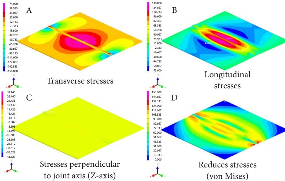
Fig. 6. Distribution of stresses in the welded joint analysed, sheet fixing manner – Table 3
