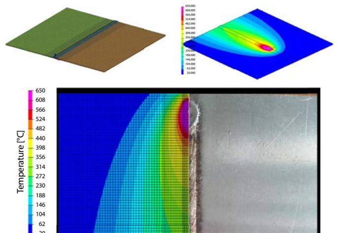
Fig. 4. Discrete model of a welded joint and the calibration of a heat source
