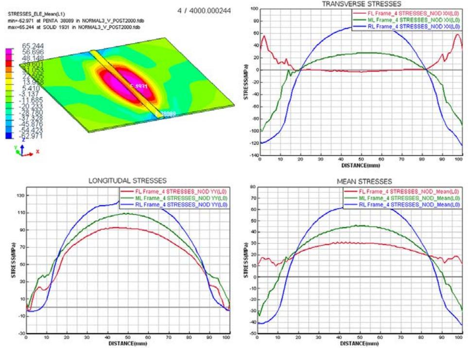
Fig. 9. Distribution of stresses on the cross-section at the half of the joint length – sheet fixing manner: variant no. 1 – Table 3
