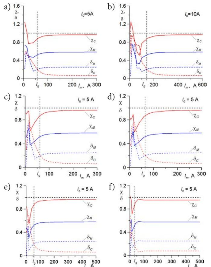
Fig. 4. Diagrams of harmonic indicators  $\chi_M(I_m)$  and  $\chi_C(I_m)$  and measures of deviation  $\delta_M(I_m)$  and  $\delta_C(I_m)$  from Mayr and Cassie models
