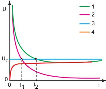
Fig. 2. Static current-voltage characteristics of (1 – a real intensively cooled arc; 2 – an arc described by the Mayr model; 3 – an arc described by the Cassie mode; 4 – a real thermally insulated arc)
