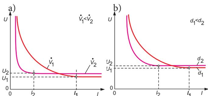
Fig. 1. Current-voltage characteristics of an electric arc
