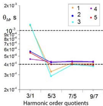
Fig. 5. Effect of the quotient of harmonic numbers  $(2k+1)/(2k-1)$  on the determination of the time constant  $\theta_M$
