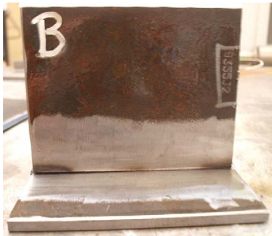
Fig. 7. Workpieces with a small amount of the anti-spatter substance in the interface
