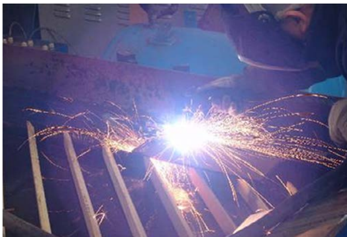
Fig.20. Manual plasma cutting process
