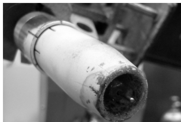
Fig. 13. Nozzle and contact tube with the anti-spatter coating after 5-minute long welding.
