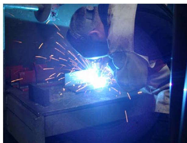
Fig. 11. MAG welding in steel – visible significant spatter.
