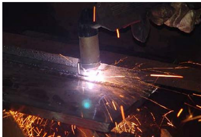
Fig.20. Manual plasma cutting process
