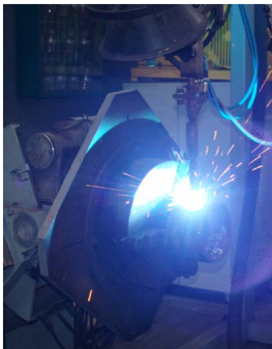
Fig. 14. MAG overlay welding of pipes
