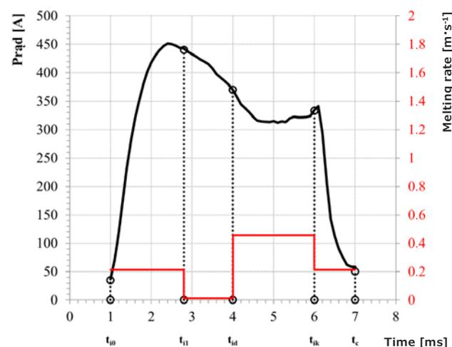
Fig. 6. Average melting rates dependent on the physical state of the filler metal wire tip during the time of current impulse
