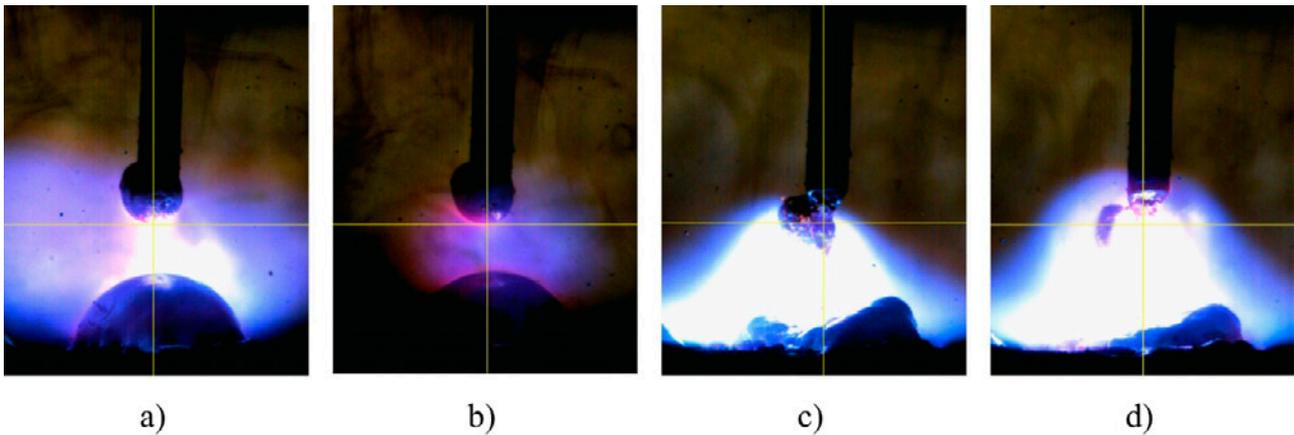
**Fig. 3** Transfer of metal in the double-pulse process: a) heating impulse, b) transition phase between working impulse, c) phase of separation impulse current up-slope and the reduction of the area between the drop and the filler metal wire and d) separation of the drop during the final impulse phase
