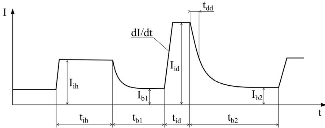
**Fig. 2** Proposed current waveform of the double impulse process melting the filler metal wire and separating the drop of liquid metal
