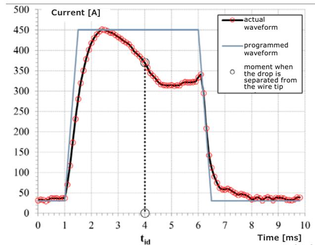
**Fig. 4** Actual and declared welding power source impulse current waveforms of voltage output characteristic in the pulsed current phase
