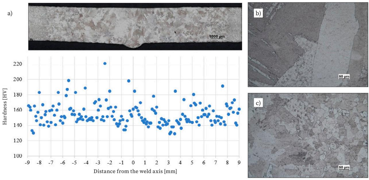
Fig. 2. Joint A: a) joint cross-section and hardness distribution, b) weld microstructure and c) HAZ microstructure
