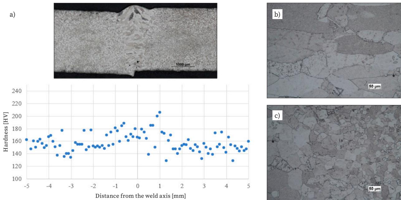
Fig. 5. Joint D: a) joint cross-section and hardness distribution, b) weld microstructure and c) HAZ microstructure
