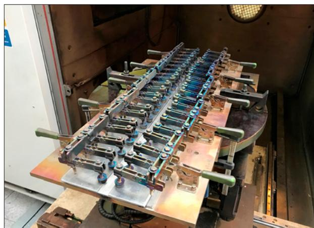
**Fig. 1.** Test sheets fixed before welding
