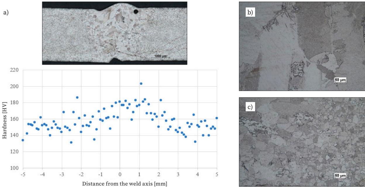
Fig. 4. Joint C: a) joint cross-section and hardness distribution, b) weld microstructure and c) HAZ microstructure
