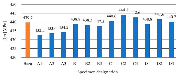
Fig. 6. Tensile test measurement results
