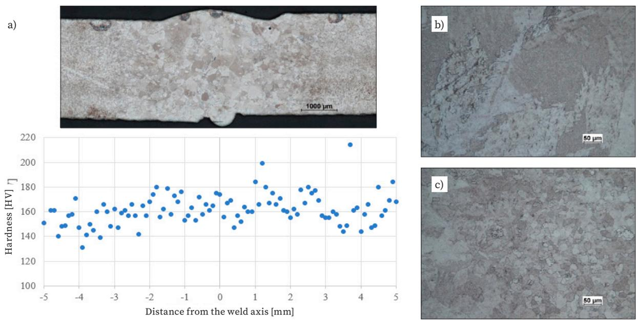
Fig. 3. Joint B: a) joint cross-section and hardness distribution, b) weld microstructure and c) HAZ microstructure
