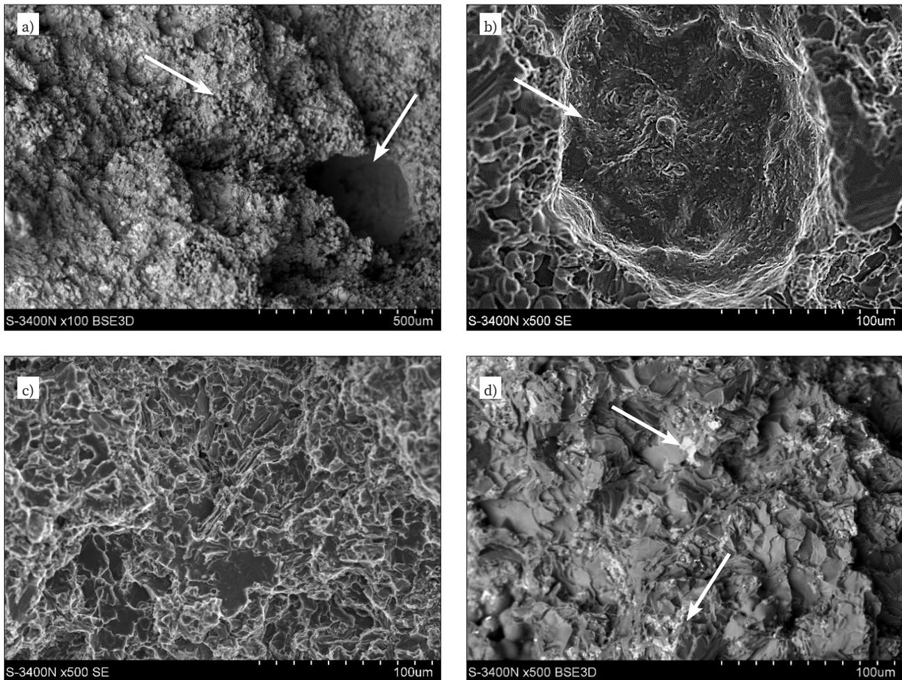
**Fig. 5.** Fracture surfaces in the EN AC-Al Si<sub>9</sub>Cu<sub>3</sub>(Fe) alloy, SEM: a) gas pore surrounded by shrinkage porosity observed on the fracture of the modified alloy, b) gas pore observed on the fracture of the unmodified alloy, c) brittleness of the unmodified alloy and d) intermetallic phase particles on the fracture surface of the modified alloy
