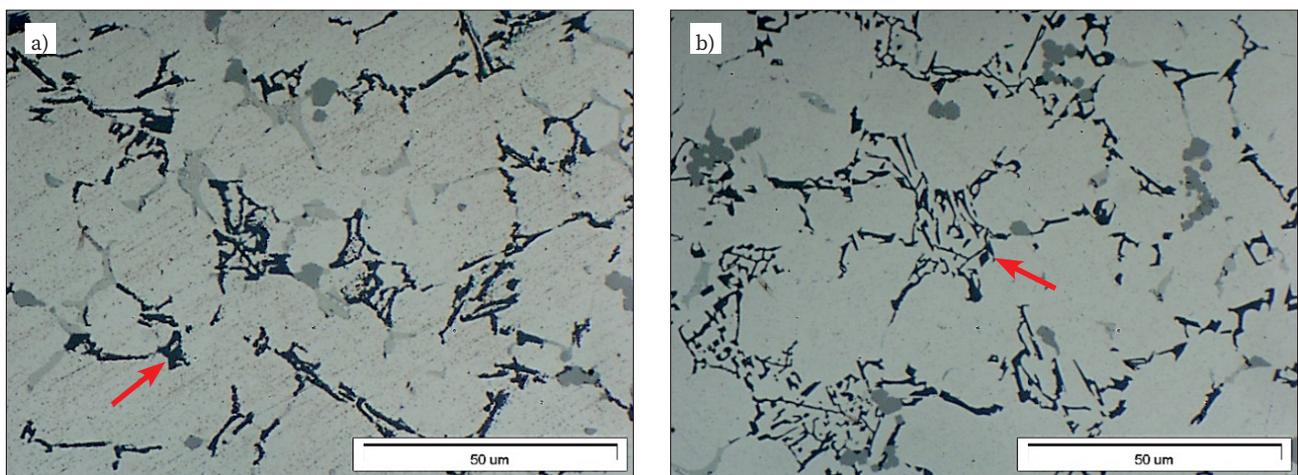
Fig. 3. AlSi9Cu3(Fe) alloy microstructure after Sr-based modification, LM: a) 40 ppm Sr addition, b) 130 ppm Sr addition
