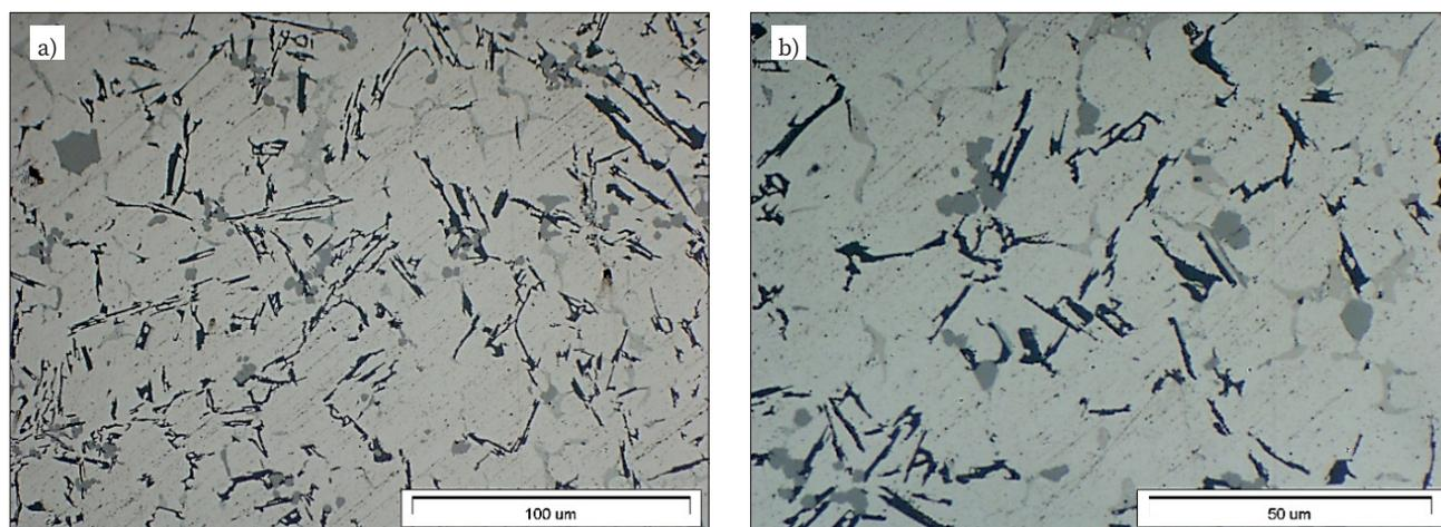
**Fig. 1.** Unmodified AlSi9Cu3(Fe) alloy microstructure, LM
