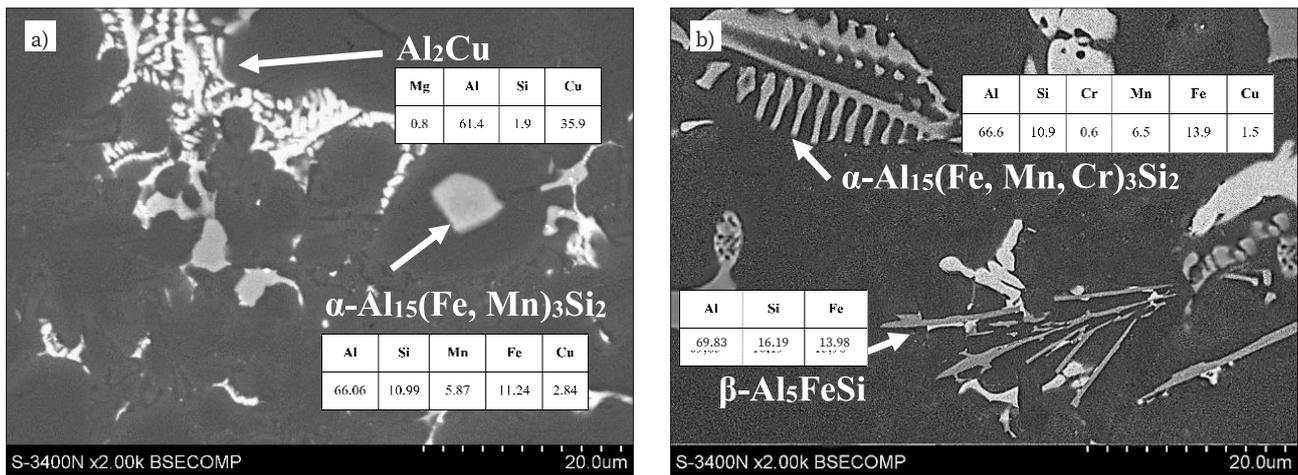
Fig. 2. Intermetallic phases in the structure of the AlSi9Cu3(Fe) alloy (at%), SEM
