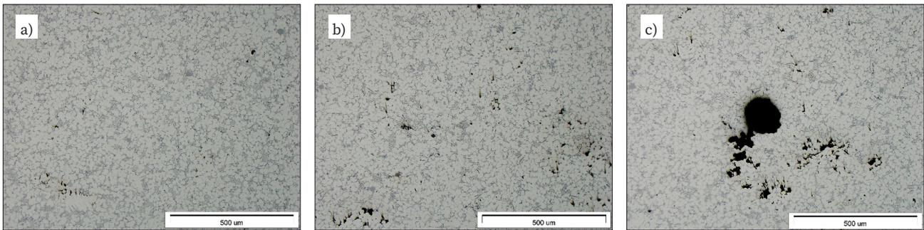
**Fig. 4.** Porosity in the AlSi9Cu3(Fe) alloy, LM: a) unmodified alloy, b) 40 ppm Sr addition and c) 130 ppm Sr addition
