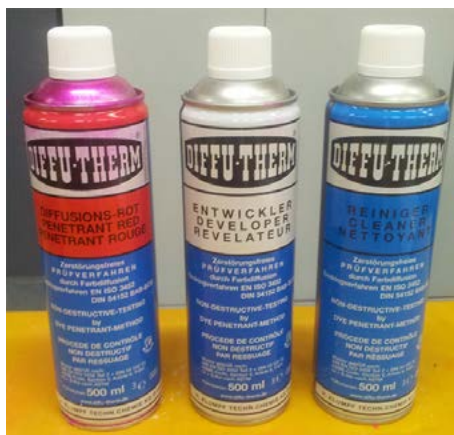
Fig. 3. Set of aerosols "Diffu - Therm" used in the liquid-penetrant inspection of plates with simulated pores
