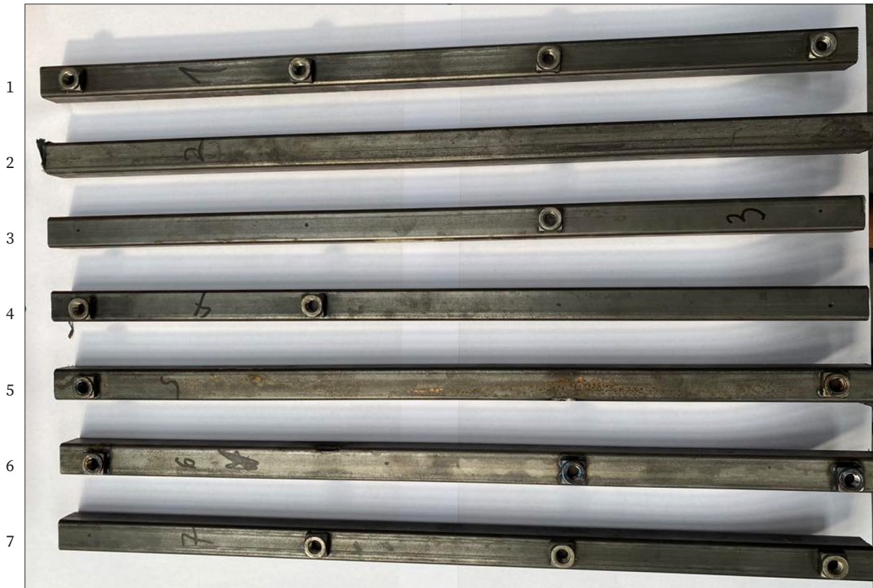
Fig. 9. Test specimens: 1 – standard specimen with all nuts welded to the section, 2 – section without nuts (welded to it), 3 – section with nut no. 3 (welded to the section), 4 – section with nuts nos. 1 and 2 (welded to the section), 5 – section with nuts nos. 1 and 4 (welded to the section), 6 – section without nut no. 2 and 7 – section without nut no. 1
