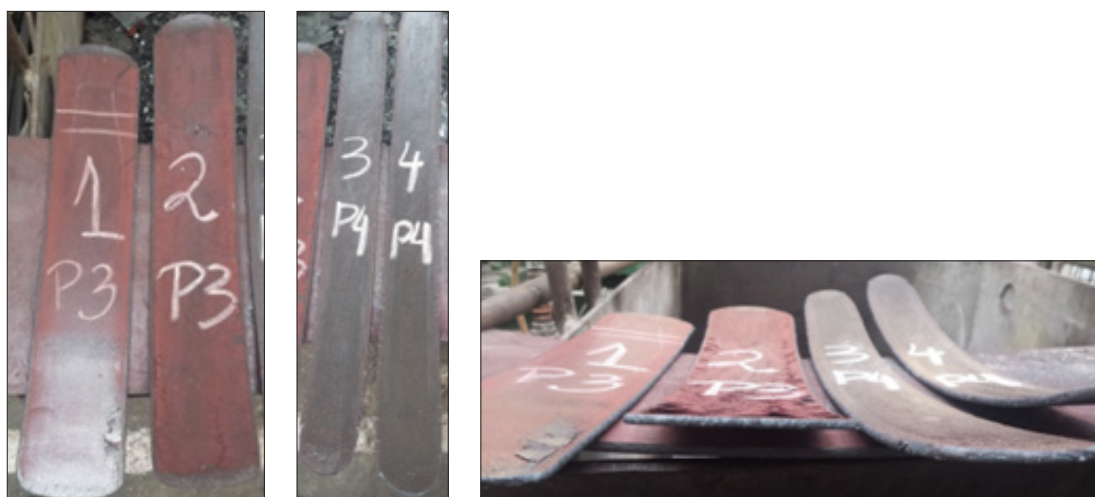
Fig. 2. Photographs of layered flat bars after hot rolling in the semi-industrial simulation line (module B-LPS)
