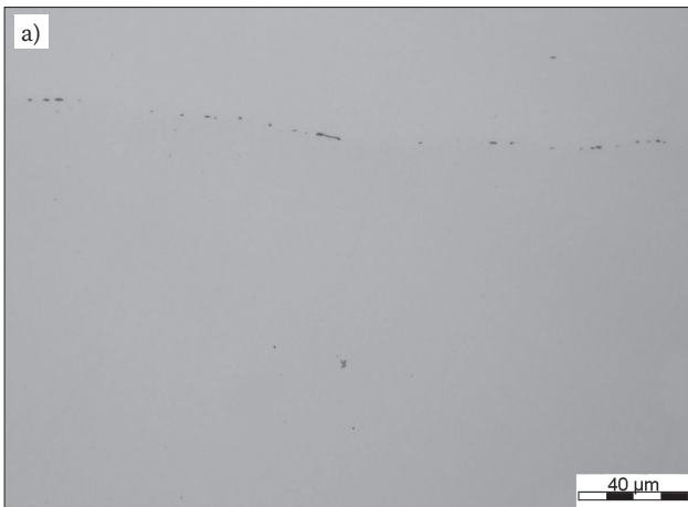
Fig. 4. Microstructure of the layered plate made of steel S235JR and steel X20Cr13 (variant 2): a) unetched specimen (LM) and b) specimen etched with Nital (SEM)
