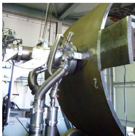
Fig. 7. Example of an electron beam welding machine with a local chamber [8]
