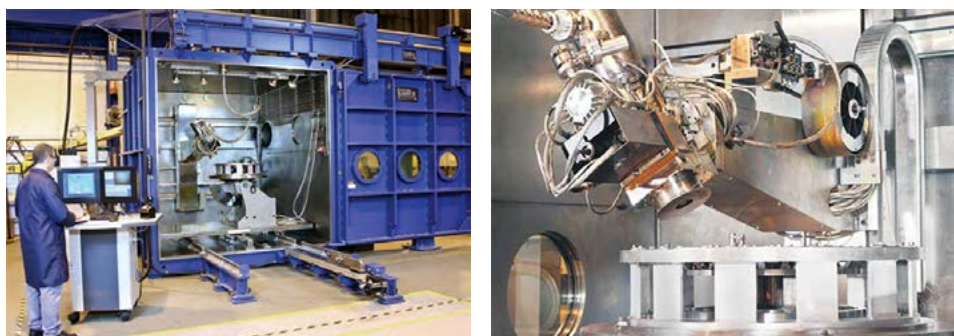
Fig. 6. Example of a Sciaky-manufactured electron beam welding machine with a moving electron gun [7]
