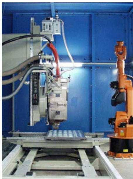
Fig. 8. Non-vacuum electron beam welding machine, P=24.5 kW, U=175kV [9]
