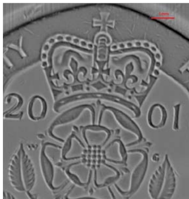
Fig. 11. Example of an image recorded using back-scattered electrons [4]
