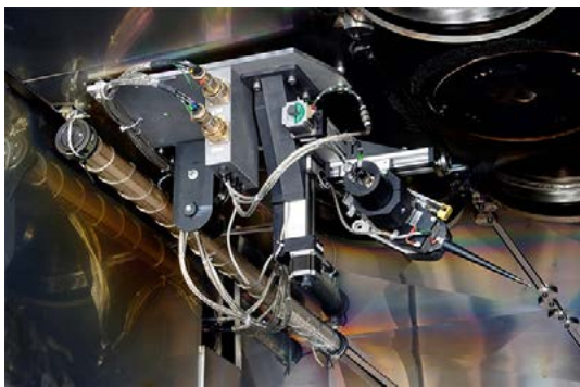
Fig. 15. Electron beam welding electrode wire feeding system [4]
