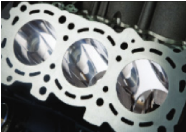
Fig. 4. Gliding surface obtained on the cylindrical surface of the 63 AMG engine cylinder
