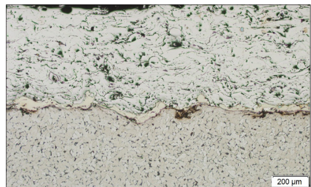
Fig. 15. EuTronic Arc 595 coating magnified 100×
